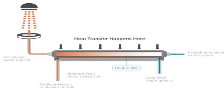
Figure 5. EcoDrain heat exchanger for use with the shower water [10].
