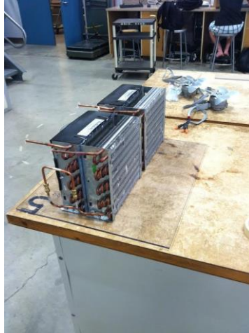
Figure 26. Evaporator Layout (Two rear evaporators providing the main cooling and two forward evaporators functioning as pre-cooling devices)
