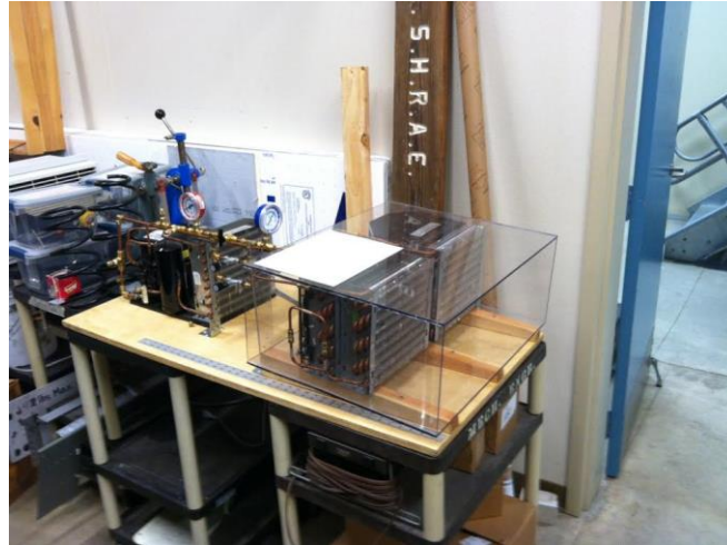
Figure 28. Assembly with condensing unit on the far left and duct with enclosed evaporators on the right.
