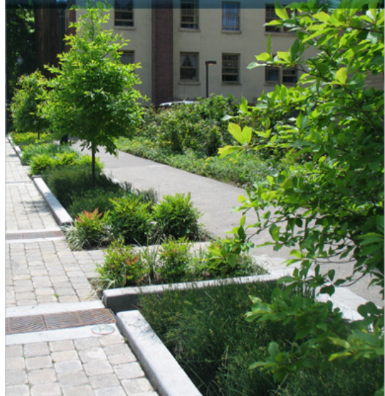
Figure 2.9: Example of landscaping that act as a low-impact drainage solution by filtering the rain water flows before it hits the main pipes.
