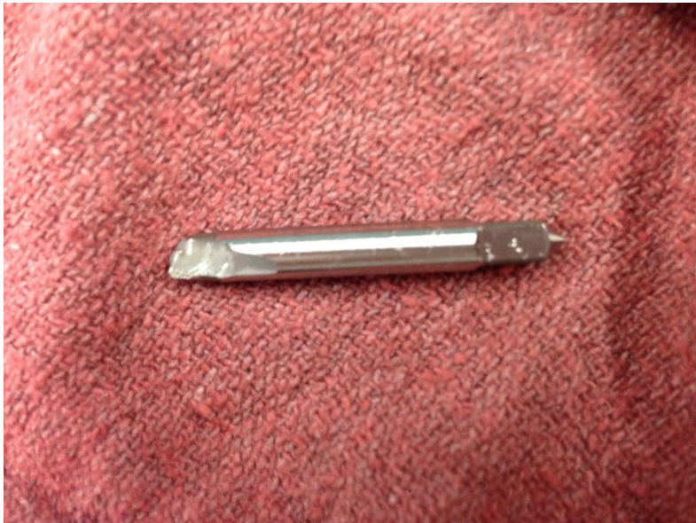
Figure 1: A broken tap due to incorrect tap replacement
