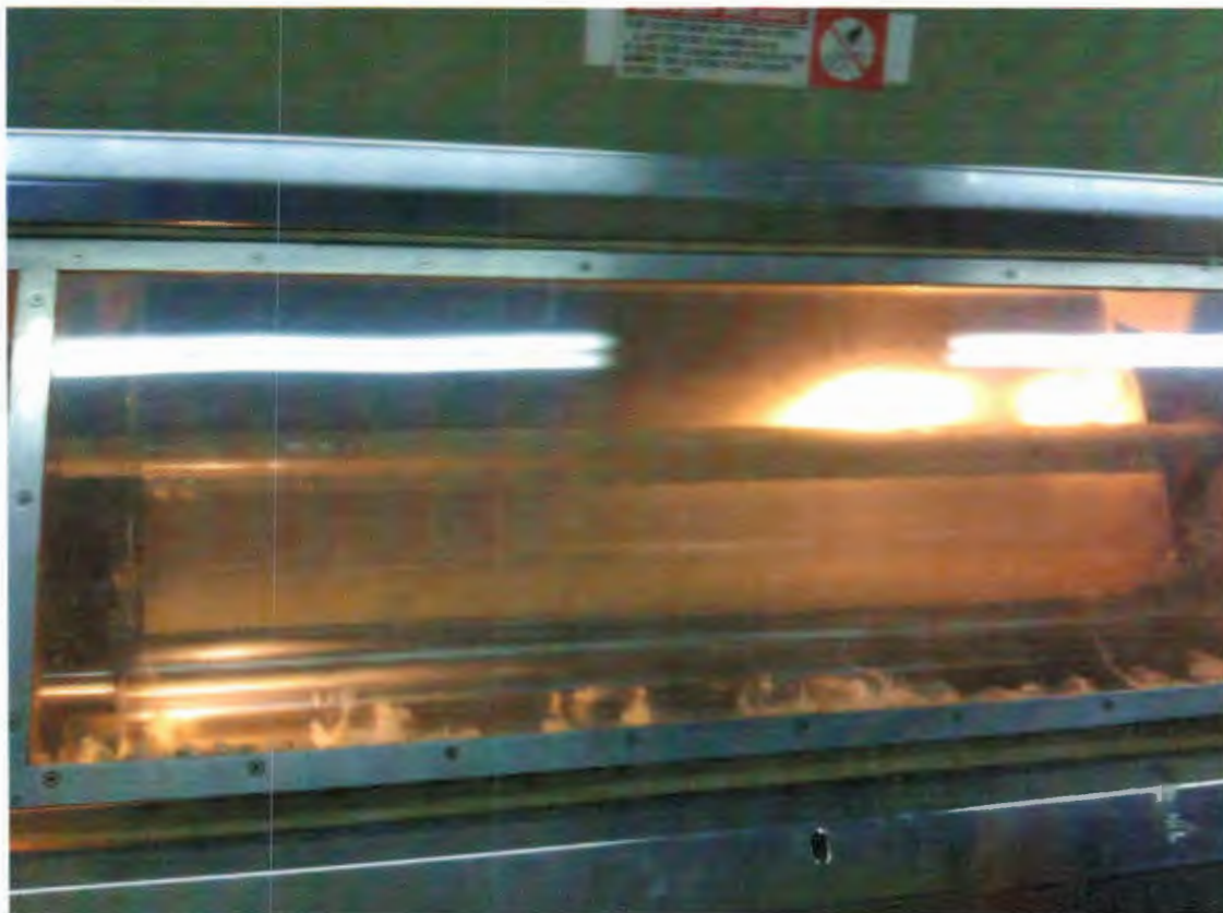
Figure 5. Cotton seed being separated from cotton fiber.
