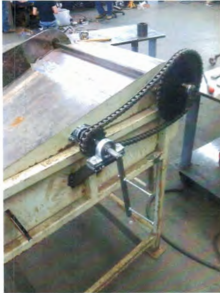
Figure 15. Complete gear reduction assembly.
