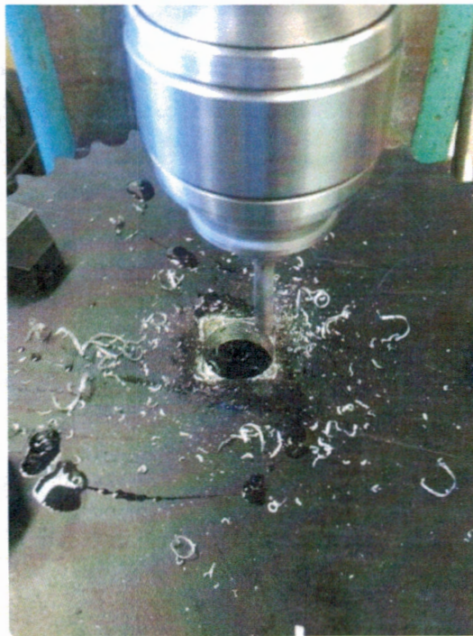
Figure 13. Milling square bore on driven sprocket.
