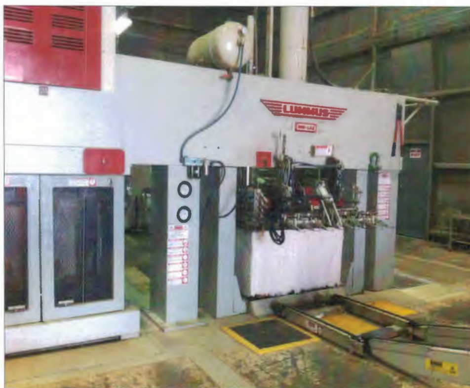
Figure 6. Cotton fiber being pressed into a bale.
