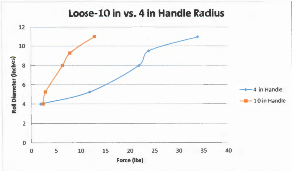
Figure 19. Comparison of 10 inch handle vs 4 inch handle in Slop position.
