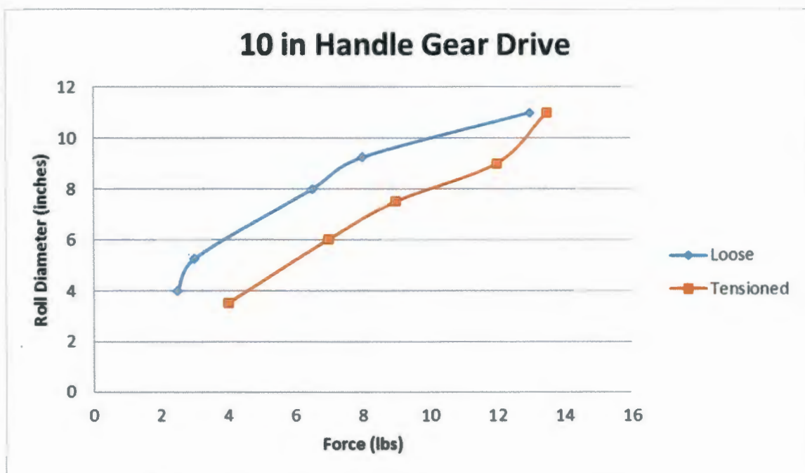
Figure 18. Relationship of force and roll diameter.
