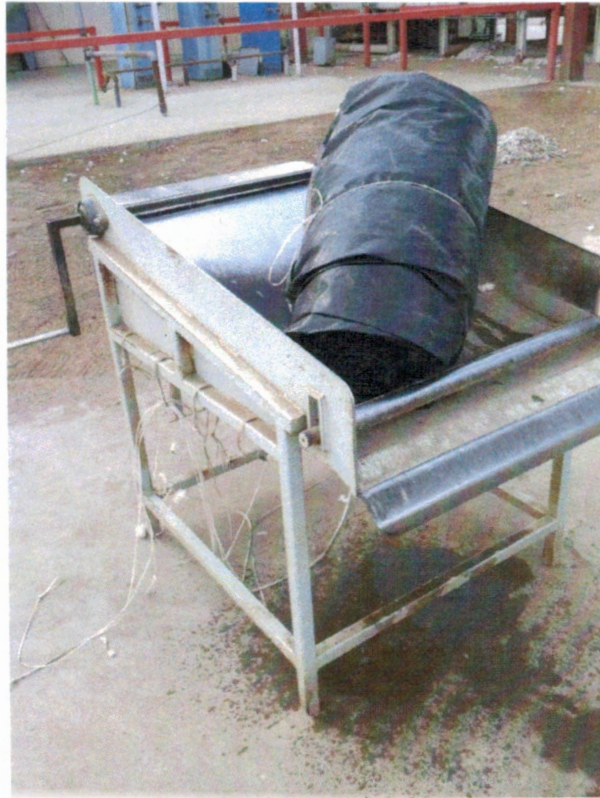
Figure 1. Cotton module tarp roller currently used and a rolled tarp
