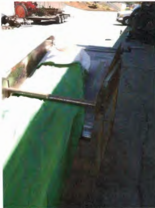
Figure 9. "Tensioned" testing position for tarp rolling.
