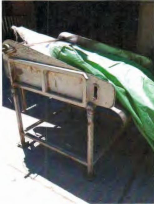
Figure 8. "Loose" testing position for tarp rolling.
