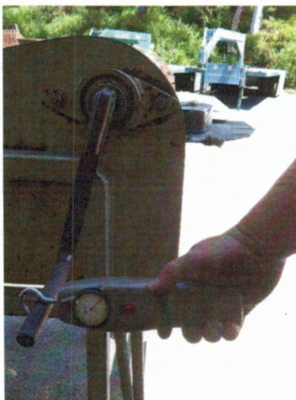
Figure 7. Analog Force Gauge used to measure torque.
