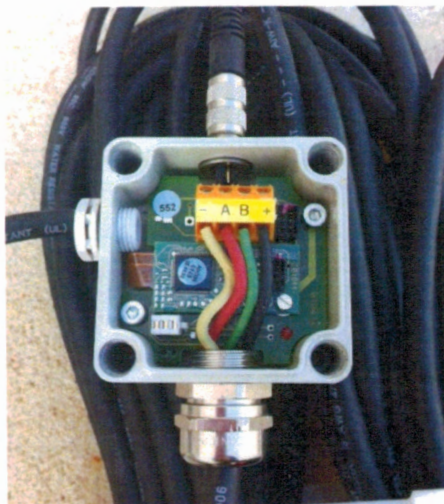
Figure 24: Breather Box Configuration for water level sensor
