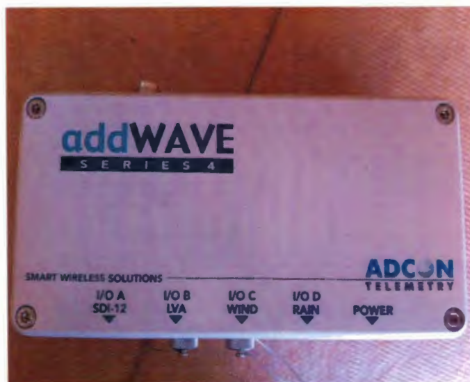
Figure 2: Remote Transmission Unit
