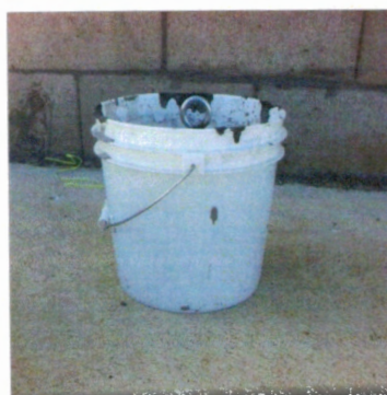
Figure 22: Concrete Weight to sink water level sensor in Nelson Reservoir
