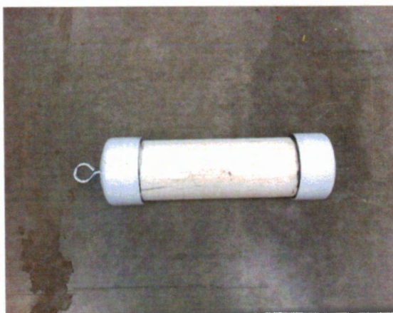
Figure 21: PVC Float for Nelson Reservoir water level sensor
