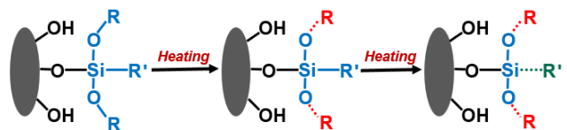
FIGURE 7. Mechanism of thermal degradation of a silane grafted on silica. (During heating, the unreacted alkoxy groups marked in red will leave firstly; with further increasing temperature, the Si-R' bond of the side chain from the silane marked in green will be broken).
