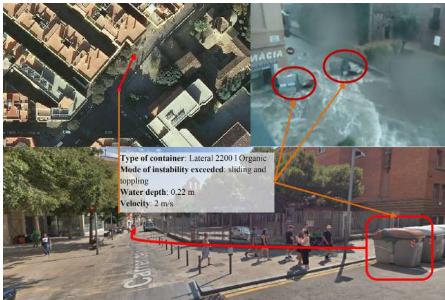
FIGURE 15 Validation of the present containers stability study based on a recorded video of the July 30, 2011 flood in Ciutat Vella district
