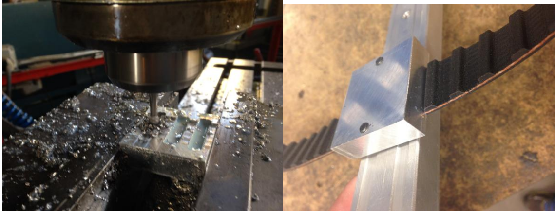
Figure 21. (Left) Belt clip being made on a mill. (Right) Belt clip attached to belt and rail.
