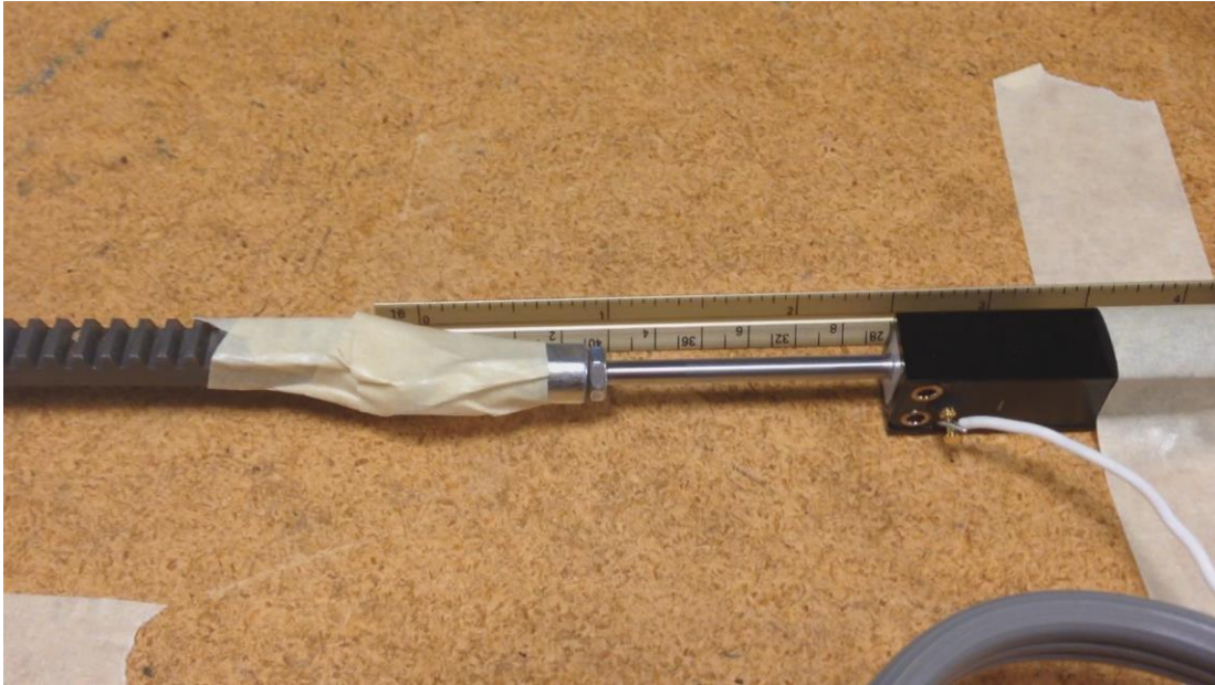
Figure 28. Correlating extension length to voltage readout.
