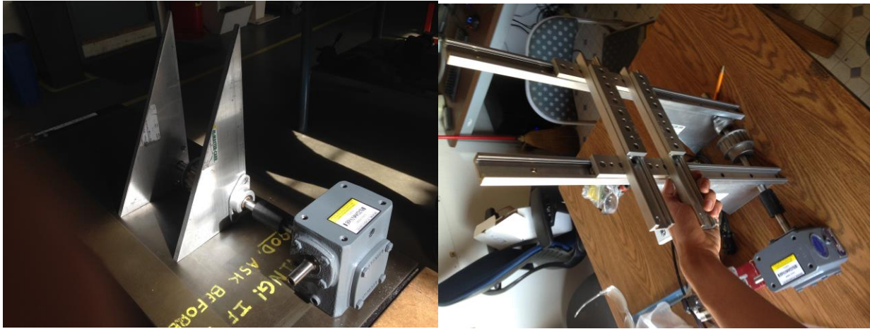
Figure 19. (Left) The angle brackets with bearings installed and drive shaft attached to the gearbox. (Right) Rail and carriage assembly attached to angle brackets and gearbox.
