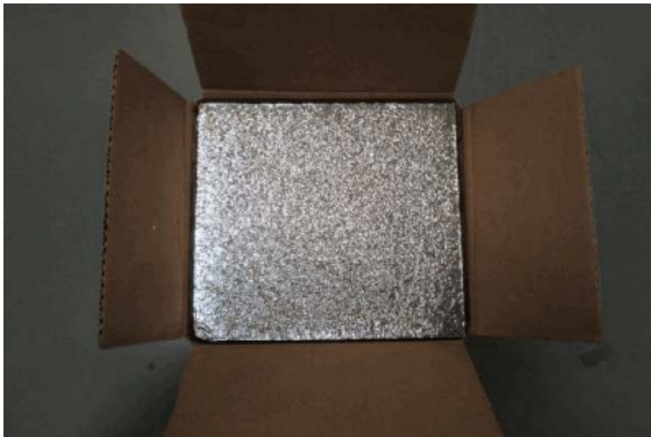
Figure 73: MAC-kage packed and sealed with the last VIP
