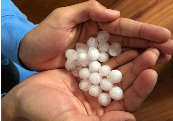
Figure 46: Frozen PCM beads filled with H 2 O
