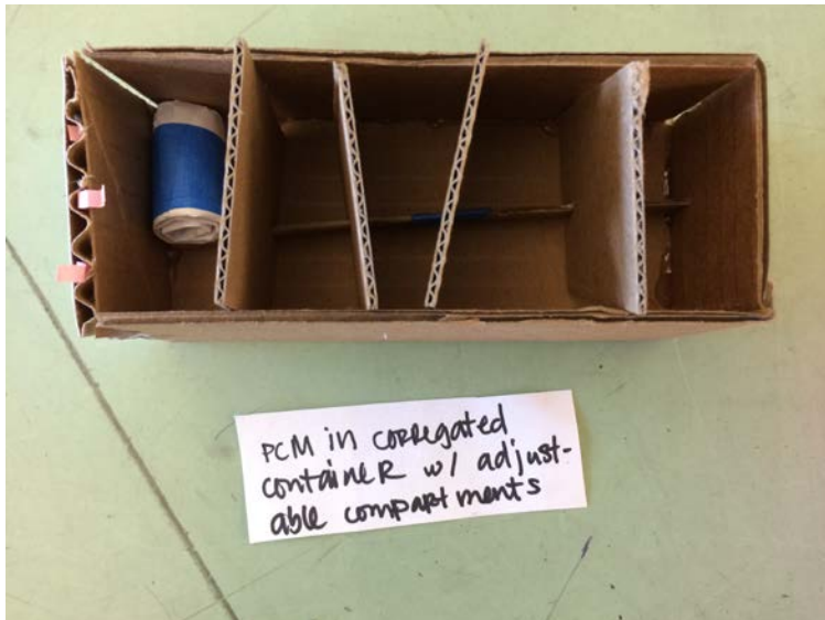
Figure 20: Versatile PCM-filled corrugated container concept
