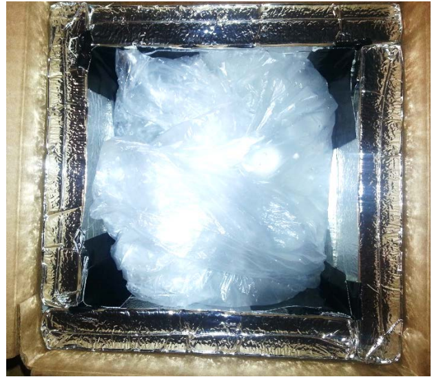
Figure 49: Bag folded over to prevent spillage
