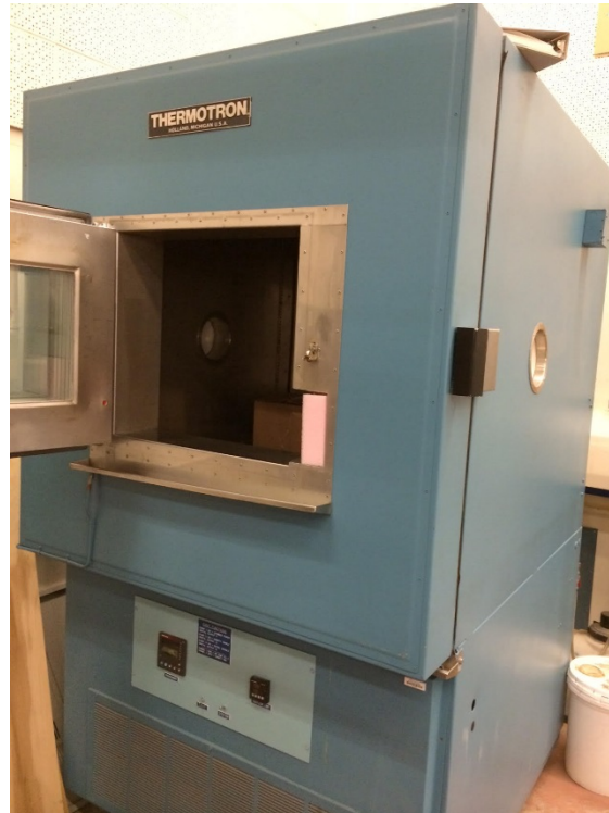
Figure 53: Packaging samples inside Thermotron test chamber
