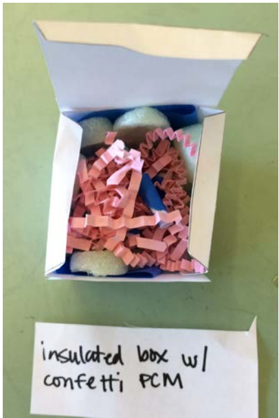
Figure 22: Particulate PCM Concept
