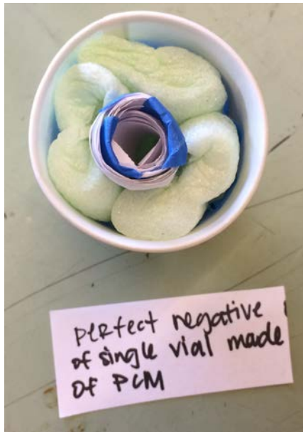
Figure 23: PCM For Individual Vials Concept
