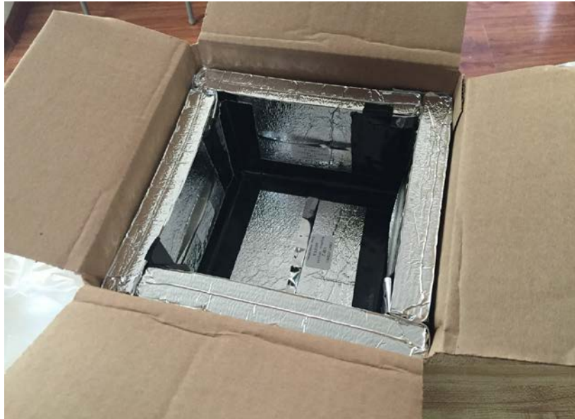
Figure 69: Assembled MAC-kage with VIP's (Lid missing from picture)
