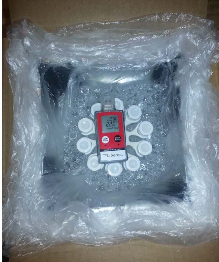
Figure 82: MAC-kage Filled with PCM, Vials, and a Temperature Monitor Ready to be shipped.
