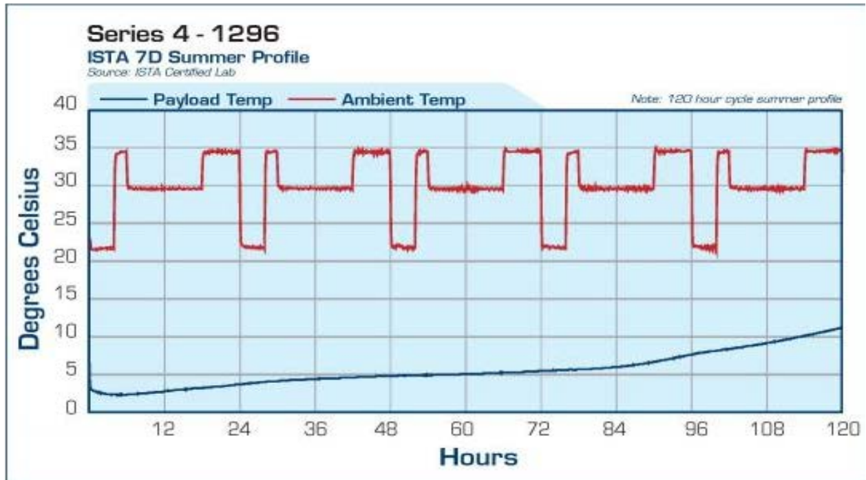
Figure 54: Credo Cube Temperature Loading ("Series 4 1296 [Credo Cube]", 2014)
