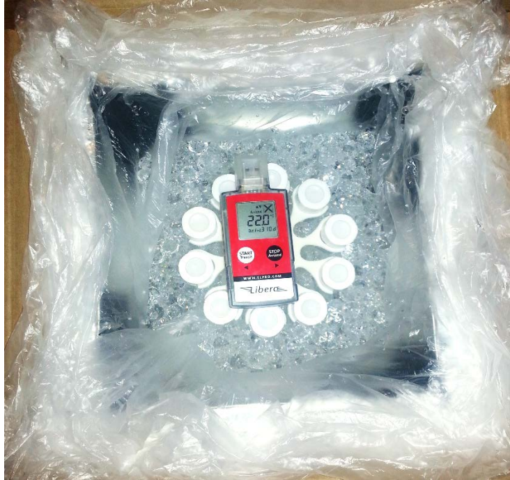
Figure 52: Visual Test for Temperature Monitor Inside the MAC-kage
