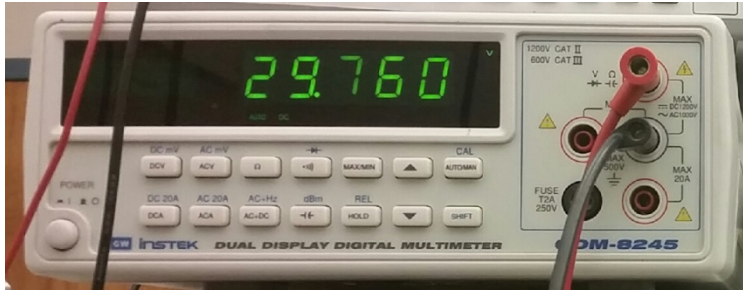
Figure 5-6: Output Voltage @ 330k ohm feedback resistor
