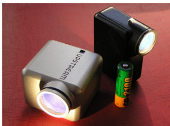
Figure 4.1 The Pocket Projection device produced by Upstream Company (Source: WEB_2, 2006)
