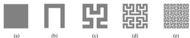
Figure 1 Hilbert iteration configurations (a) original, (b) first iteration, (c) second iteration, (d) third iteration, and (e) fourth iteration
