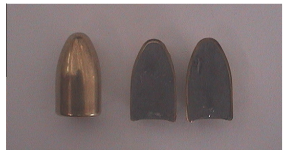
Fig. 4. Projectile of the 9 mm × 19 Parabellum cartridge and its cross sections.
