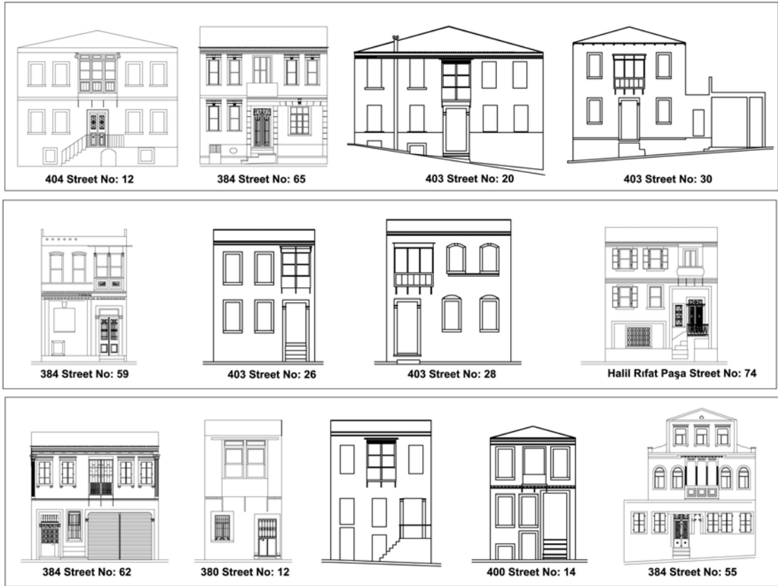
Figure 3.24. Buildings with Cumba 4
