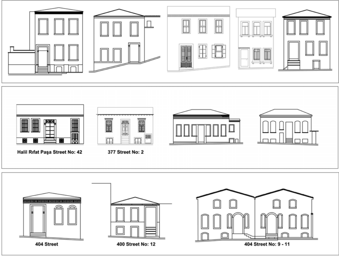
Figure 3.25. Buildings without Cumba 5
