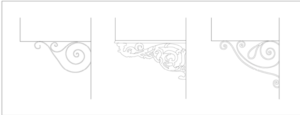
Figure 3.50. Decorative cast iron cantilevers below cumba (Source: Kaplan, et al. 2006)
