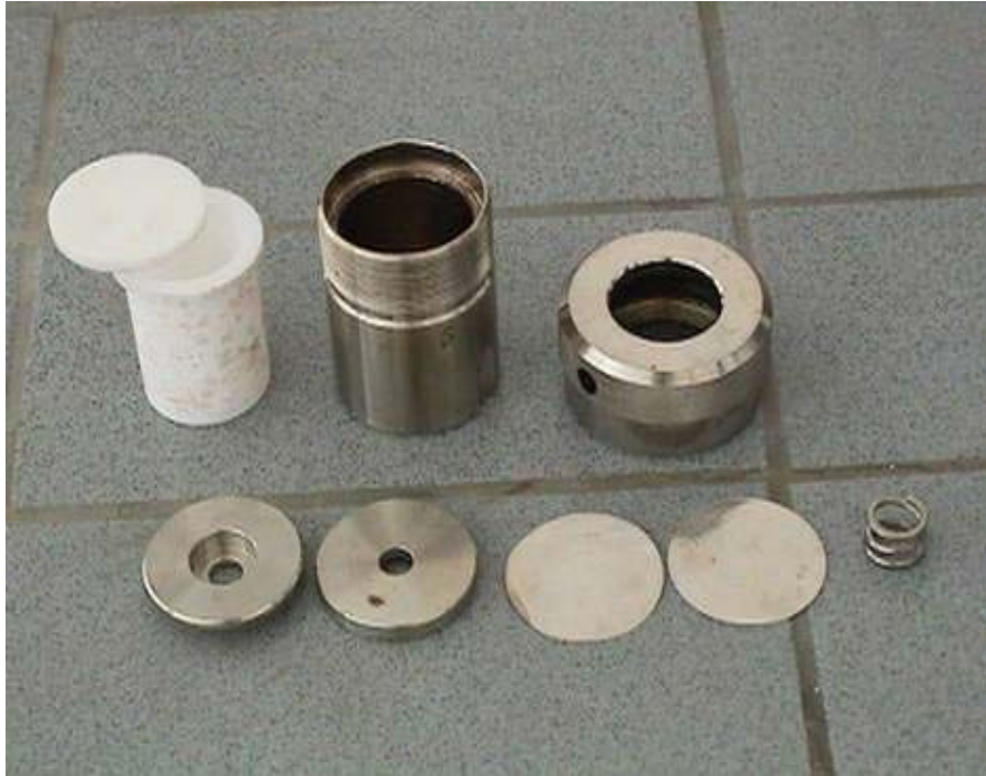
Figure 2.2. PTFE cup with cover, acid digestion bomb body, screw cap, pressure plate (upper), pressure plate (lower), corrosion and rupture discs, spring (from left to right)
