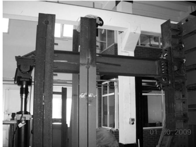
Fig. 5 Photograph of HE400AA test specimen in the test setup
