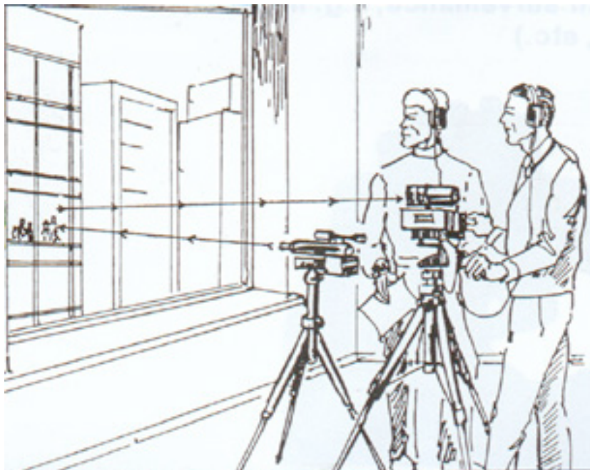
Figure 1.4. Unauthorized Listening Using Laser Microphone
