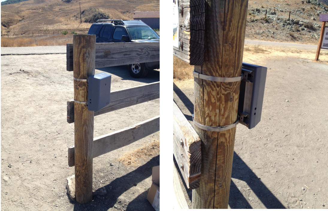
Figure 4: A pedestrian eco-counter is compact device that can detect the direction that users are moving. It counts pedestrians as they cross an invisible infrared beam emitting from the device. An example is shown at the entrance of the Johnson Ranch open space.
