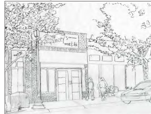
1.2a Any main street business frontages will have a small town character with minimal or no setbacks from the sidewalk to make it more pedestrian friendly.
