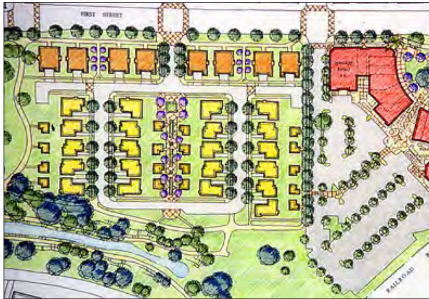
Image III: Alley-loaded granny units in Aggie Village.
