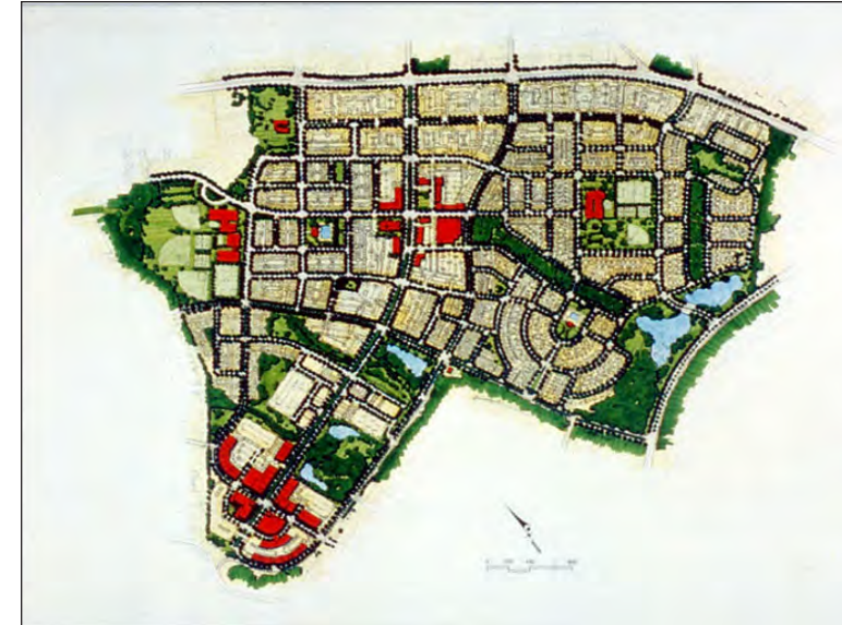
Image IV: This site plan of the King Farm development illustrates the layout of the community and its residential and commercial/public components. The orientation of the road network clearly shows how residential uses are linked to the red community/retail centers located within the three sections of the development.
