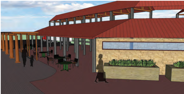
Fig. 6.23: Lightweight, modular metal structure for easy organization and expansion in the future. The structure allows trellis and spaces for seating.
