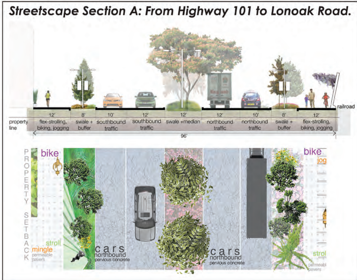
Fig. 6.8: Streetscape Section A: 12-foot median with two to four lanes design option
