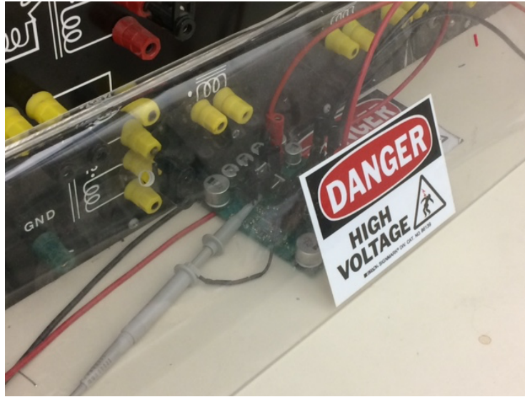
Figure 9.3 Plastic Covering over Enclosed Circuit
