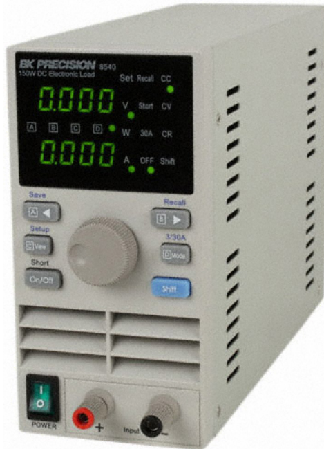
Figure 9.2 Electronic Load Used for Testing
