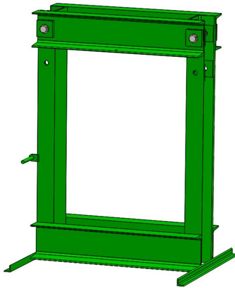
Figure 17 Final frame design, constructed of C-channels and angle iron.
