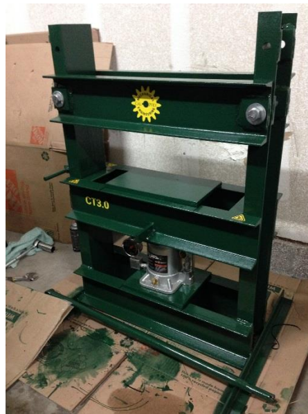
Figure 36. Final assembly of press.
