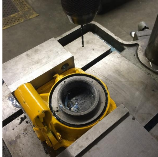
Figure 33. Tapping high pressure access hole.
