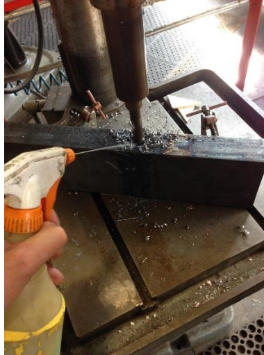
Figure 27. Cooling bit and work piece while drilling holes in c-channel.
