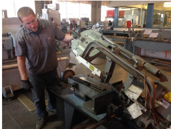
Figure 25. Cutting C-channel members with horizontal band saw.
