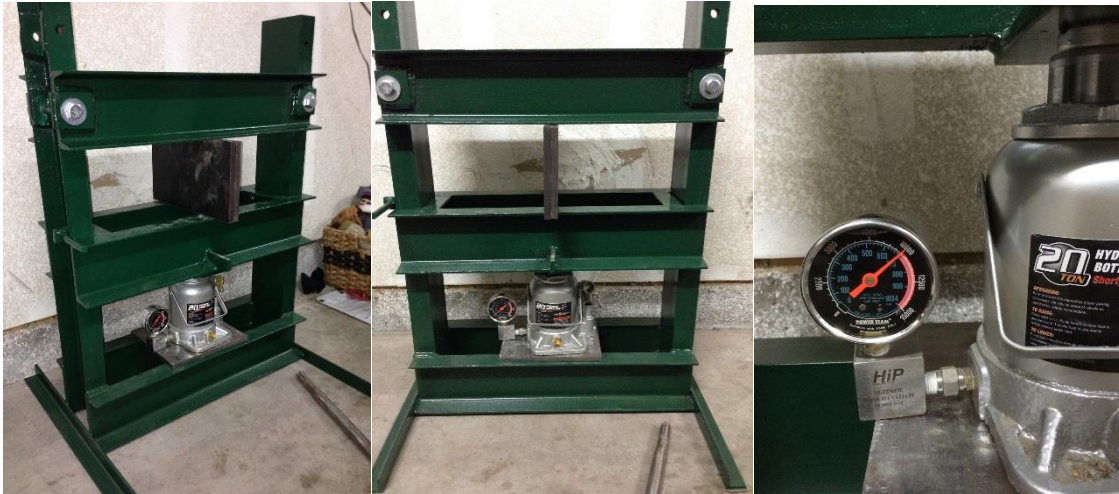
Figure 39. View of 20-ton point load testing configuration (left and center) and jack gauge during the test (right).
