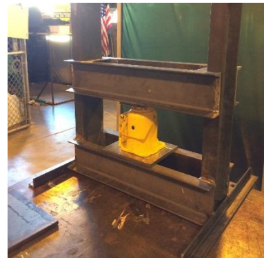
Figure 29. Checking fit of tack welded slider assembly.
