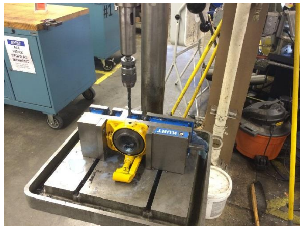
Figure 32. Hole for \frac{1}{4} " NPT tap being drilled.
