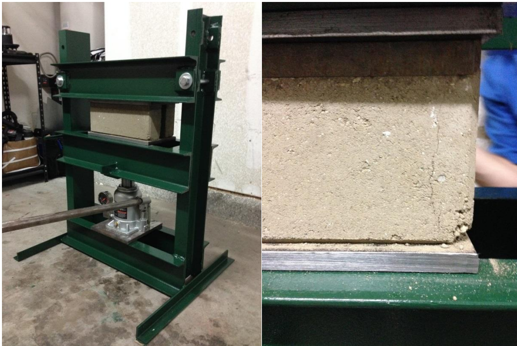
Figure 37. (Left) Press arranged in compression testing configuration. (Right) ICEB beginning to fail at corner.
