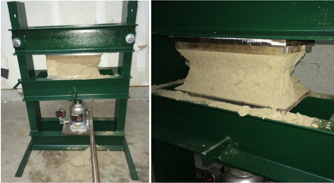
Figure 38. Total failure of ICEB.
