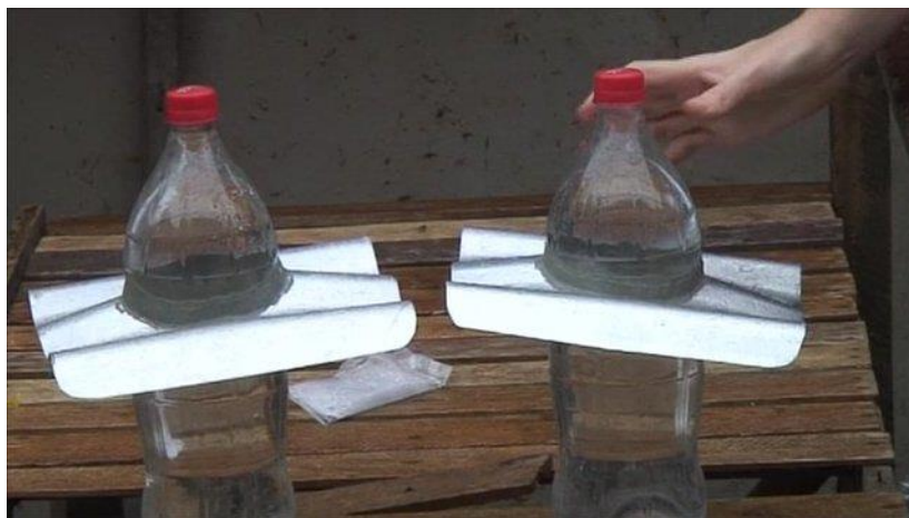
Figure 6. The water bottle light will be installed in a section of the corrugated roof
