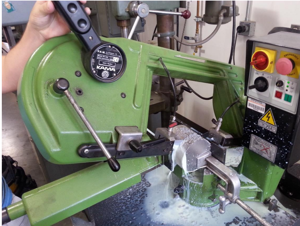
Figure 8. A horizontal saw is used to cut the stock aluminum round to length
