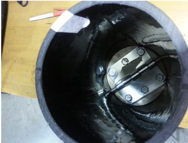
Figure 13. This picture shows how the check valve should be assembled. We used tape to indicate which flap belonged on which side. This was a result of alterations that needed to be made to the flaps due to nonuniform pipe diameter.
