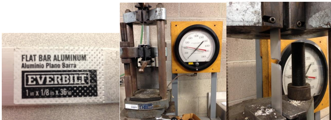
Figure 17. From left to right: bracket dimensions, tensile test setup, broken cross section
