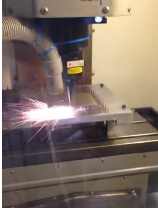
Figure 10. The valve flaps were laser cut for the prototype but would be punched with a custom die in a full production run
