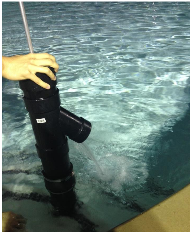
Figure 15. Pump test in PCV pool
