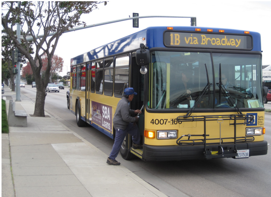
Figure 5: Passenger boarding bus from accessible landing pad.
