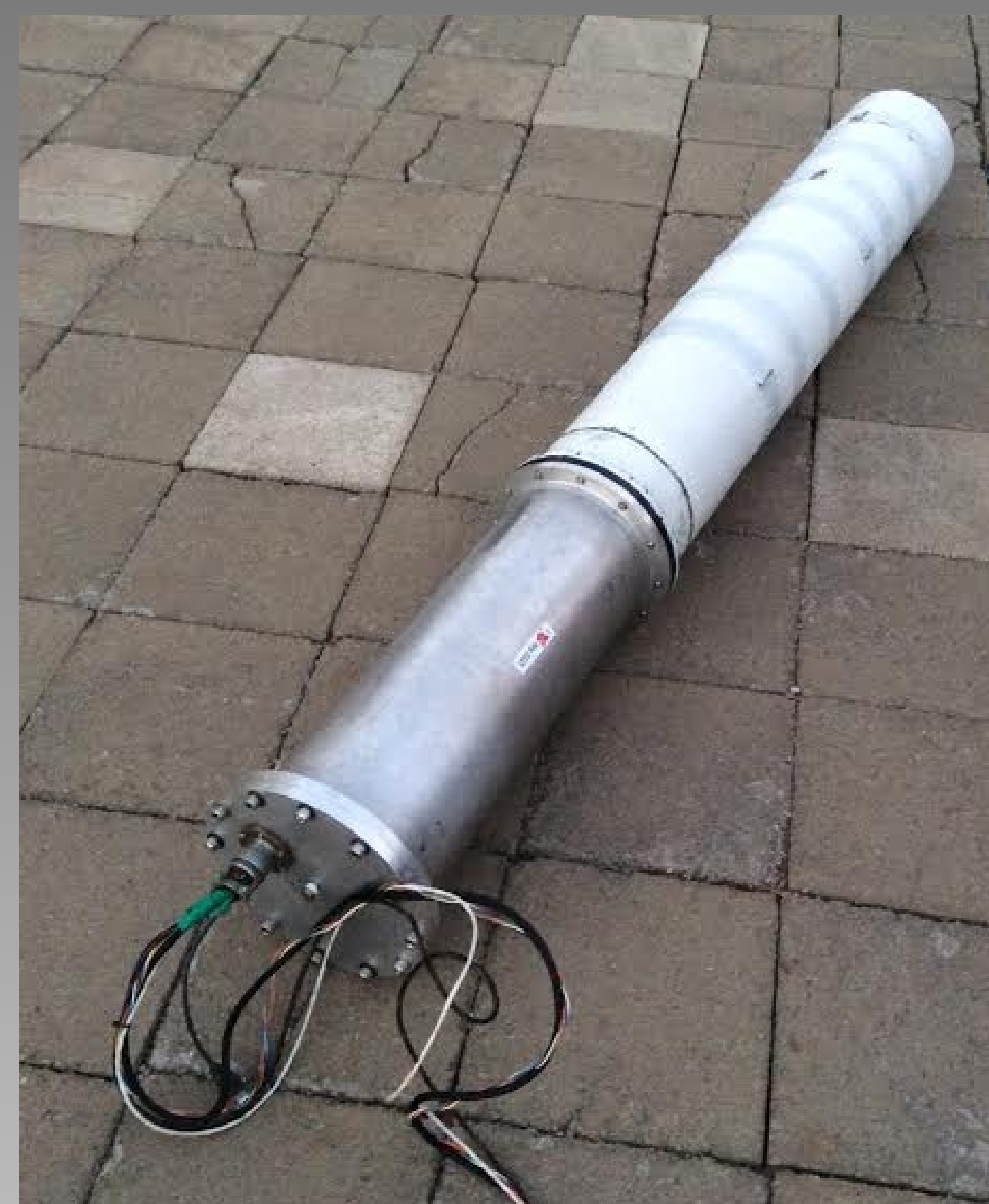
Figure 2. Complete BLAST star camera assembly contains pressure vessel and baffle.
