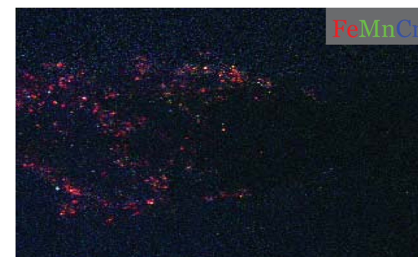
Fig 5. X-Ray Fluorescence (XRF) image of the bulb of Fig 2. Iron is imaged in red, Manganese in green, Chromium in blue.
