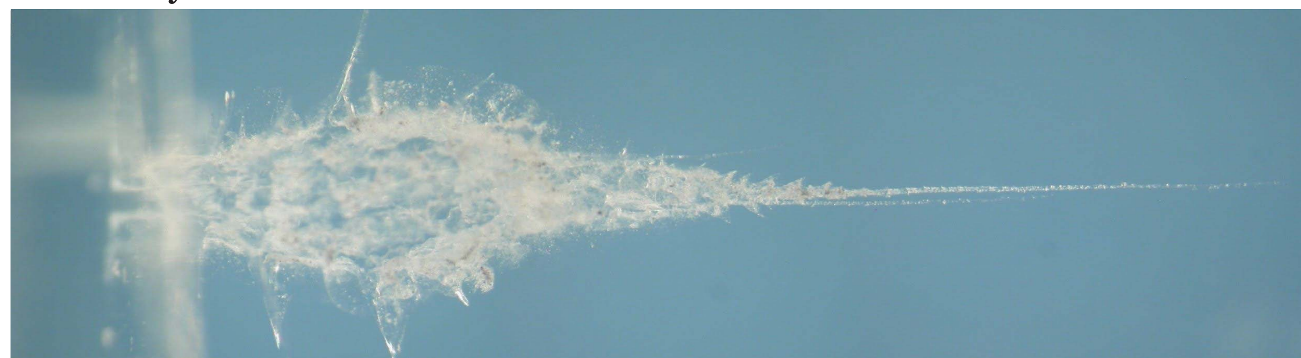
Fig 2. An optical image of an aerogel track containing a Stardust particle. Note the bulbous shape created from the high velocity impact, and the tapering ending in a terminal particle. The width of the track is ~5mm.
