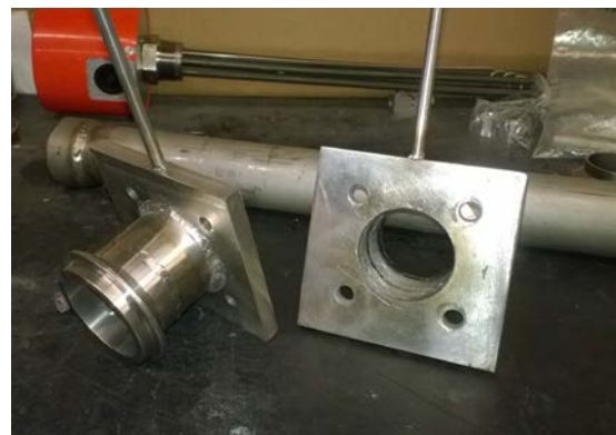
Figure 17: "Test Section" to hold orifice plates.
