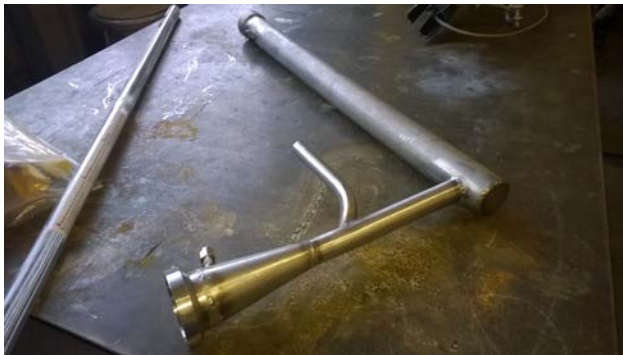
Figure 16: Welded Assembly of immersion heater housing and transfer section.
