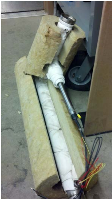
Figure 17: Flow path wrapped in insulation, both layers visible.
