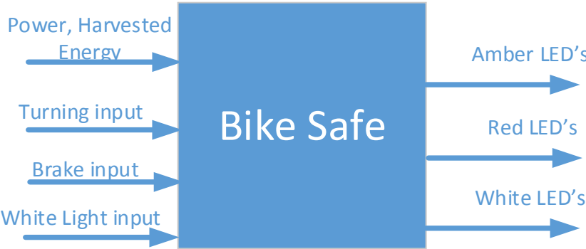
Figure 1: Level-0 Bike Turning Signal Functionality
