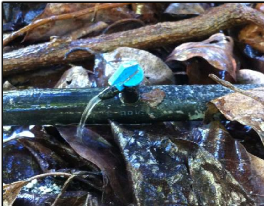
Figure 10. Example of a 2 GPH drip emitter.
