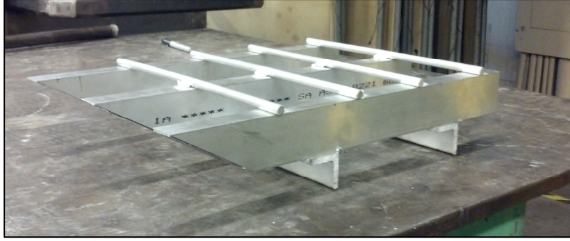
Figure 5: Angles and Rod Attached to Tubing
