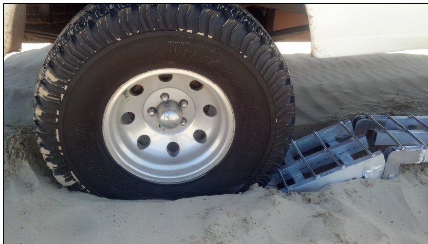
Figure 11: Utility Strip Wedged Under Tire
