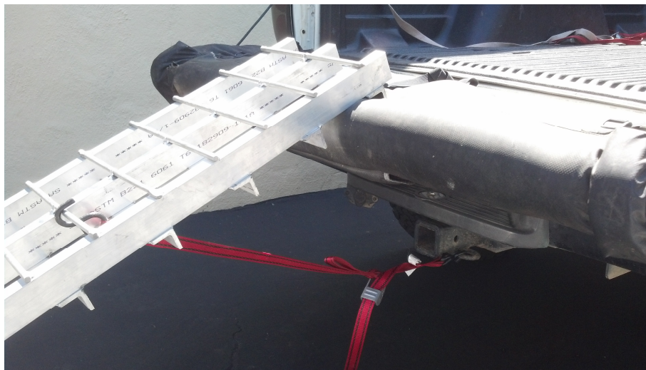
Figure 14: Tie Down Support
