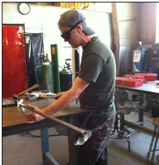
Figure 5-4 Tube Bending with an Oxyacetylene Torch
