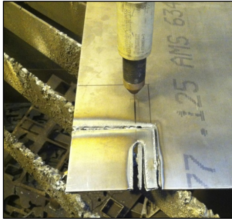
Figure 5-3 S3X Bracket Plate Cutting with an Optical Plasma Cutter
