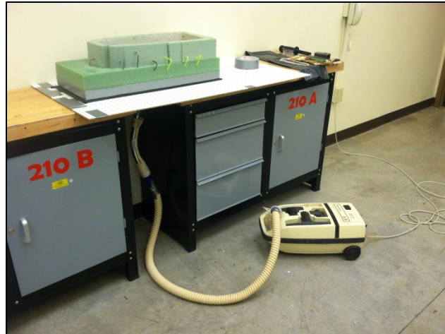
Figure 5-8 ABS Vacuum Forming Set Up
