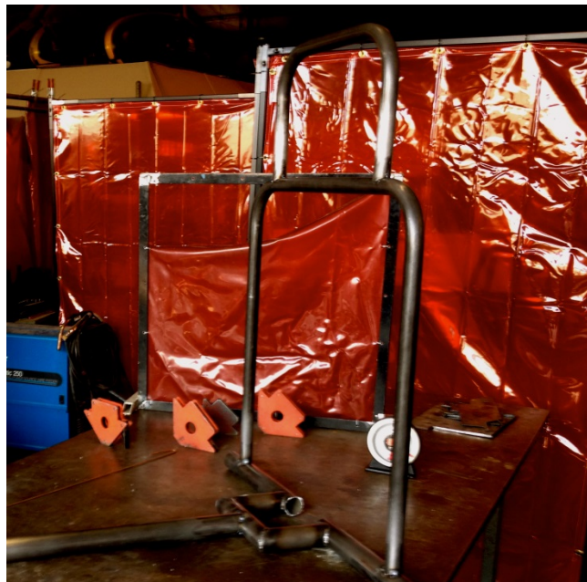
Figure 5-1 Back Bars of the Frame
