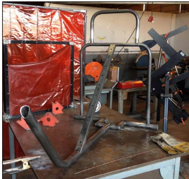
Figure 5-2 Partially Welded Frame
