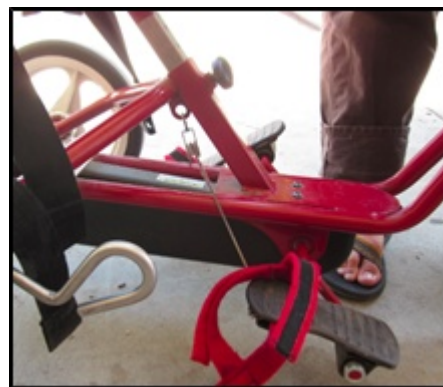
Figure 2-3 Pedal support cord on Rifton Adaptive Tricycle
