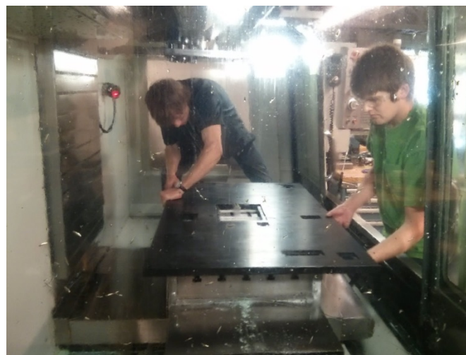
Figure 9 Loading the Tabletop inside the VF-3
