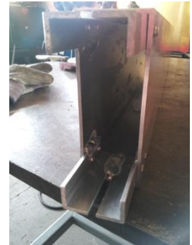
Figure 27. Angle Aluminum Welded to Track.
