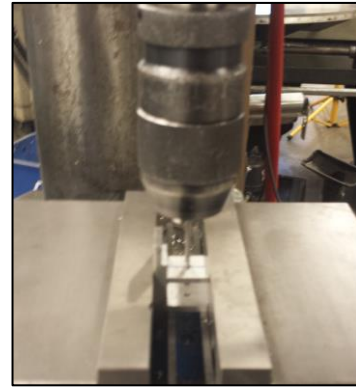
Figure 33. Vertical Drill Press creating through-holes
