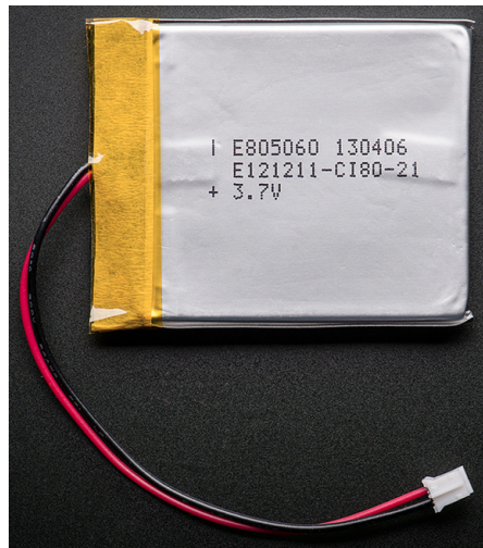
Figure 32: 2500 mAh Lithium Ion Battery [15]
