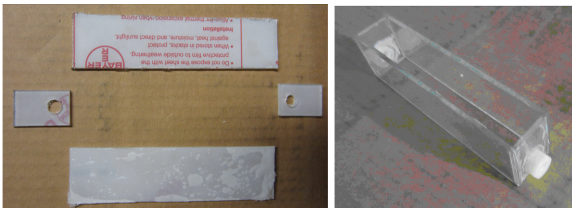
Figure 21. The calibration weight holder; parts on left, assembled on right.
