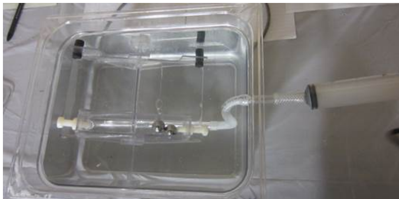
Figure 27. This shows the calibration process of the tip meters.
