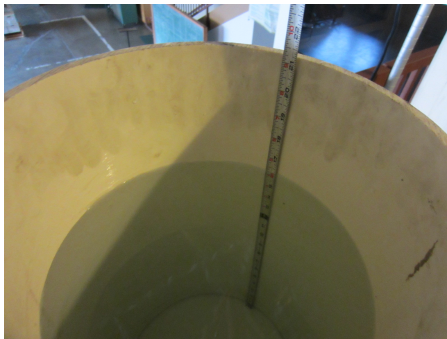
Figure 25. The digester filled with 20 L of water filled it up to 16 inches from the bottom.
