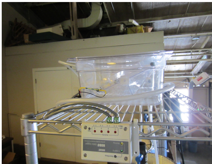
Figure 24. The tip meters fully connected to the data logger and gas ports.
