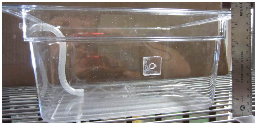
Figure 22. The water tank with 8.5 inch pipe on bottom and seesaw supports on sides. Finally the counterweight was glued onto the seesaw and it was slid into the water tank supports so it tips back and forth freely. Last the magnets and the reed switch were attached so that the switch was triggered when the meter tips, see Figure 23.
