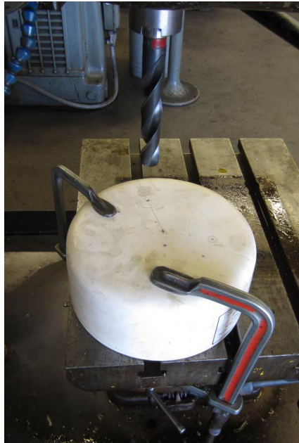
Figure 11. The lid clamped for drilling.
