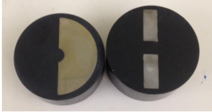
Figure 8: Mounted sample conformation (Left). McQuaid-Ehn Sample (Right).
