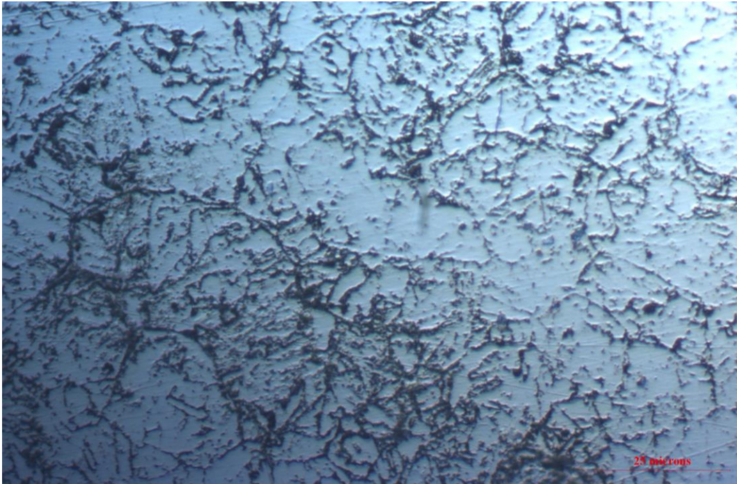
Microstructure of as-received sample.
