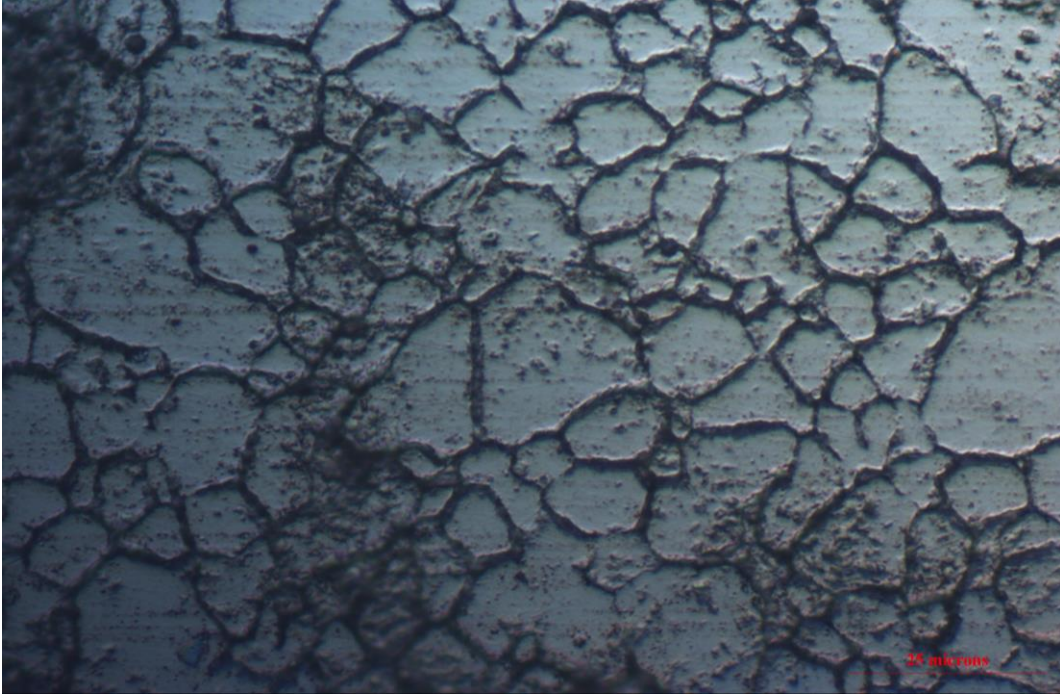
Microstructure of quenched and tempered sample (370°C for 60 minutes).
