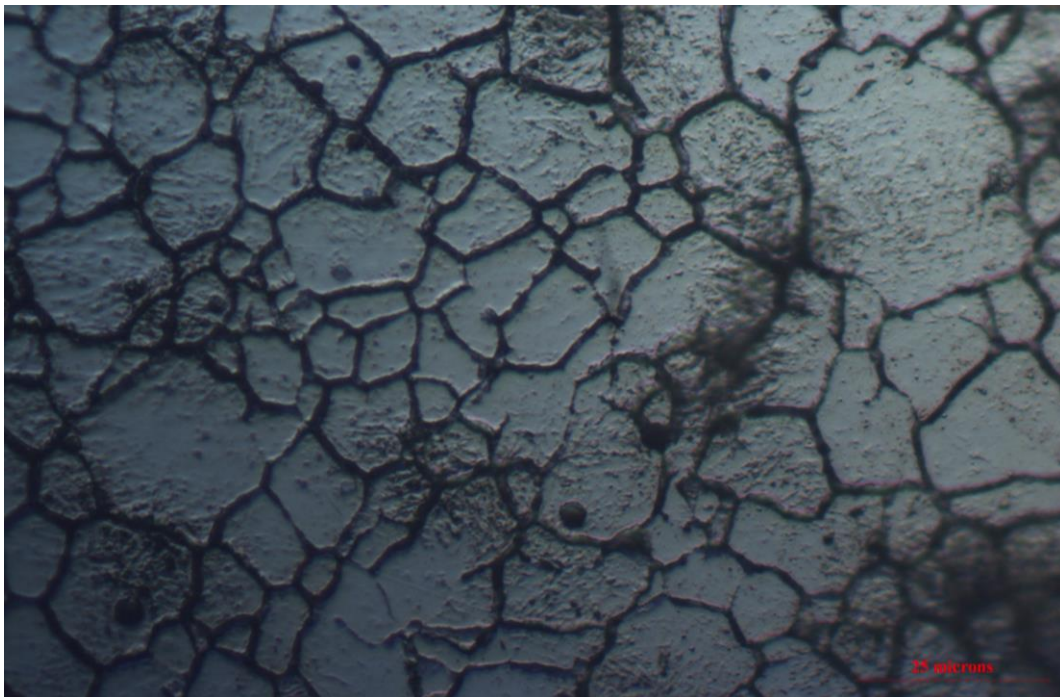
Microstructure of quenched and tempered sample (260°C for 60 minutes).
