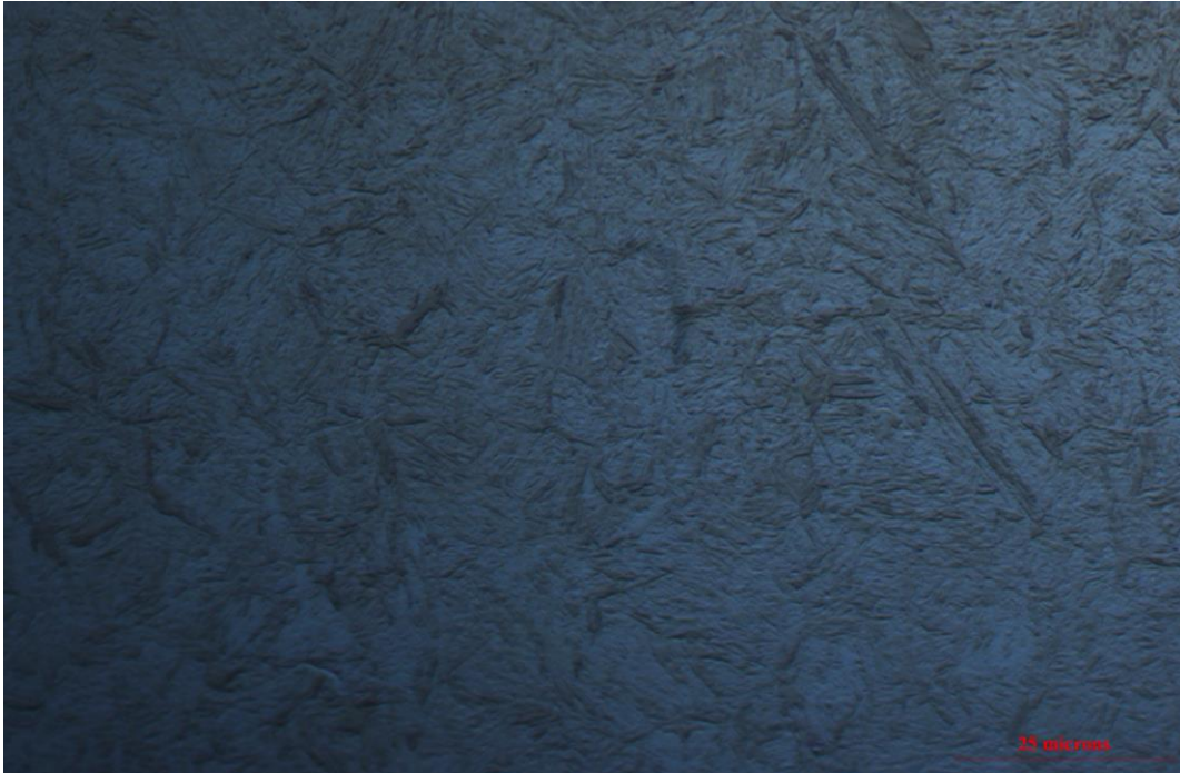
Microstructure of Hypoeutectoid sample.
