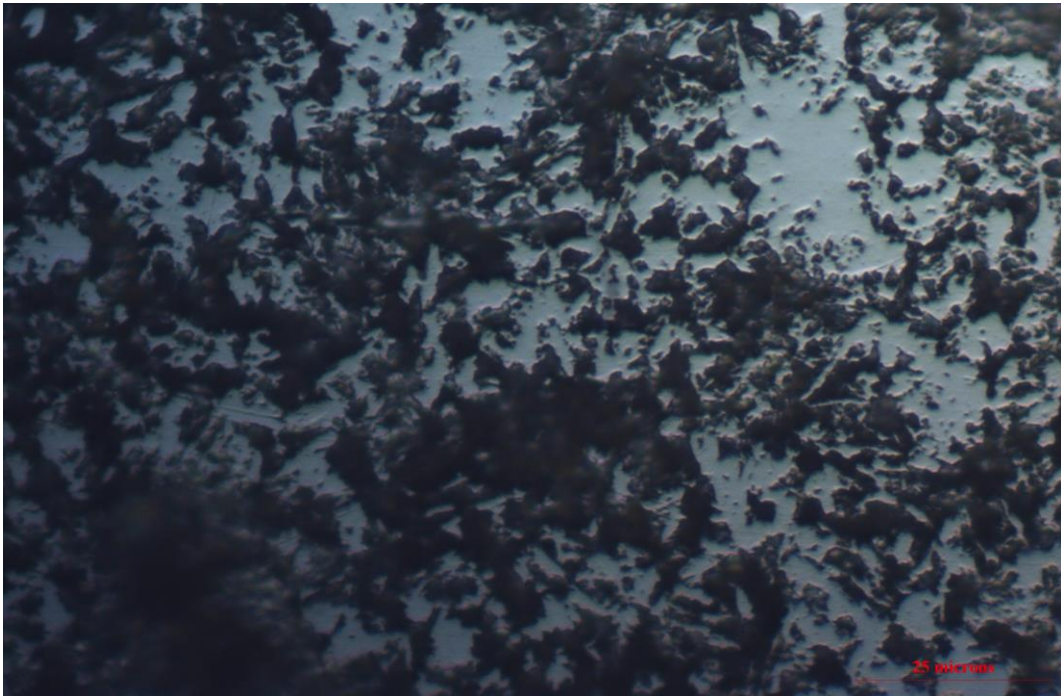
Microstructure of quenched sample.
