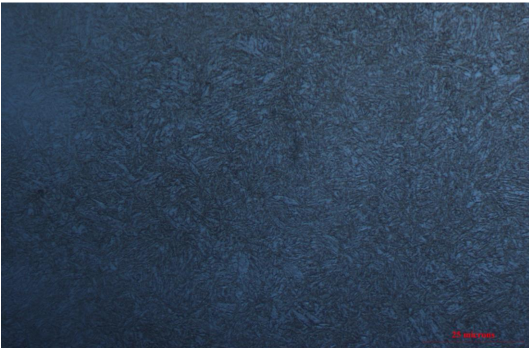
Microstructure of quenched and tempered sample (370°C for 30 minutes).
