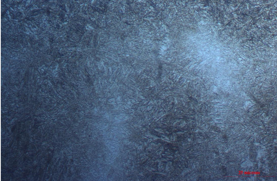
Microstructure of quenched and tempered sample (260°C for 90 minutes).
