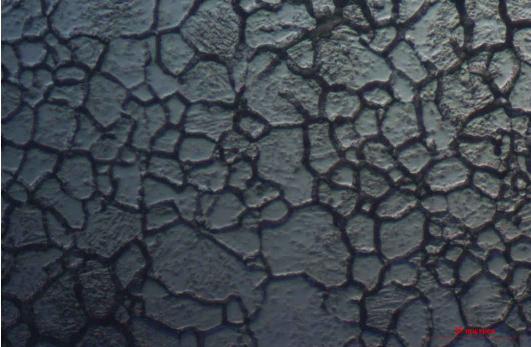
Microstructure of quenched and tempered sample (260°C for 90 minutes).
