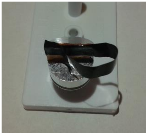
Figure 11. A sample mounted using double sided copper tape and a looped technique.
