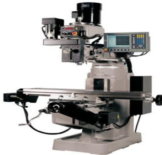
Figure 2. A Kent knee mill. Note that it does not have a chip pan or waste container.
