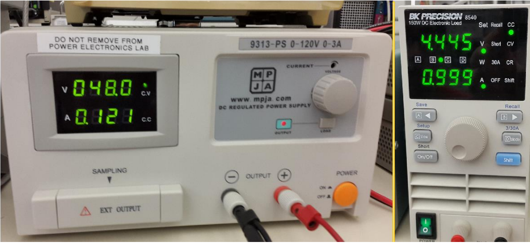
Figure 5-1: Buck Tested at 5V and 1A output
