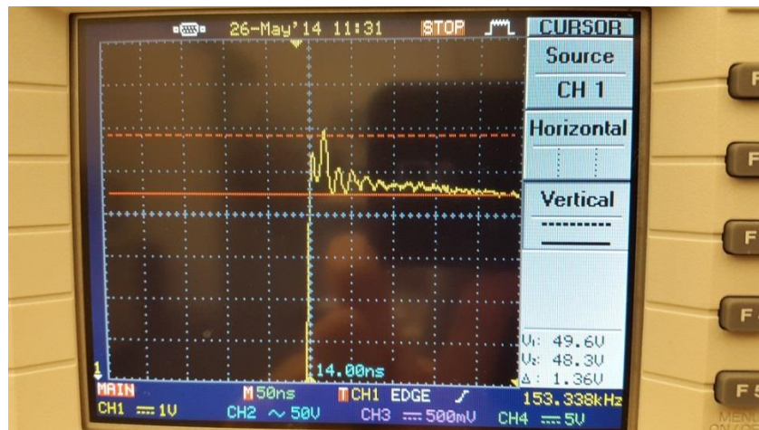
Figure 5-5 - Synchronous Switch Capture with Snubber
