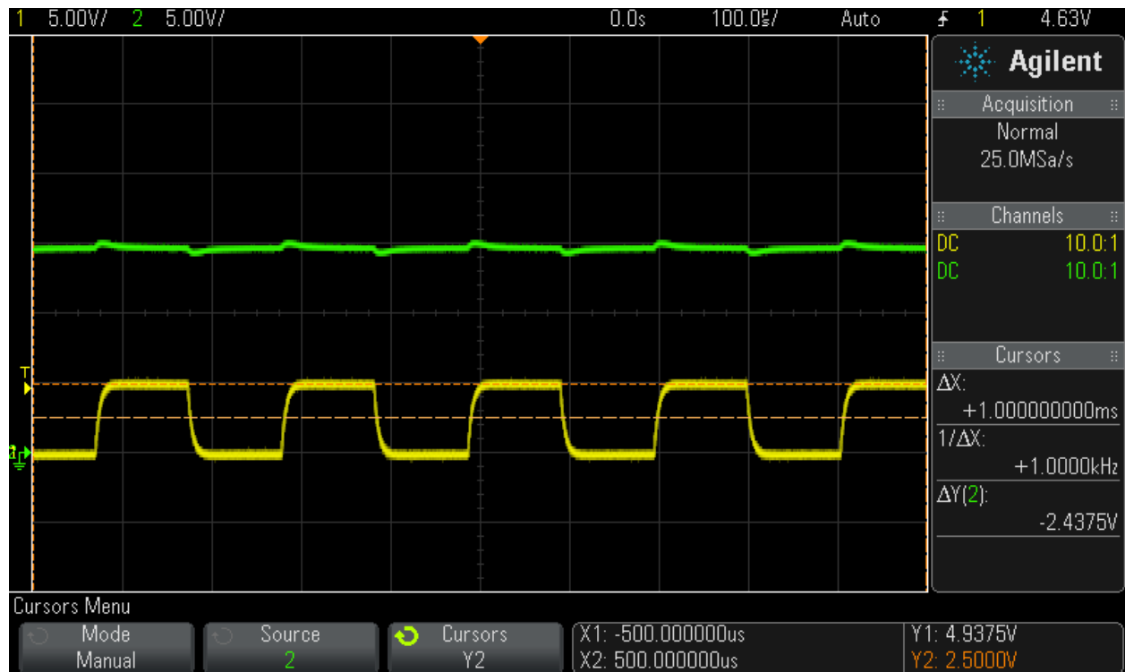
Figure 14-10: Q1 Gate Voltage vs. Drain Voltage Q2 Gate (Yellow) Drain (Green)
