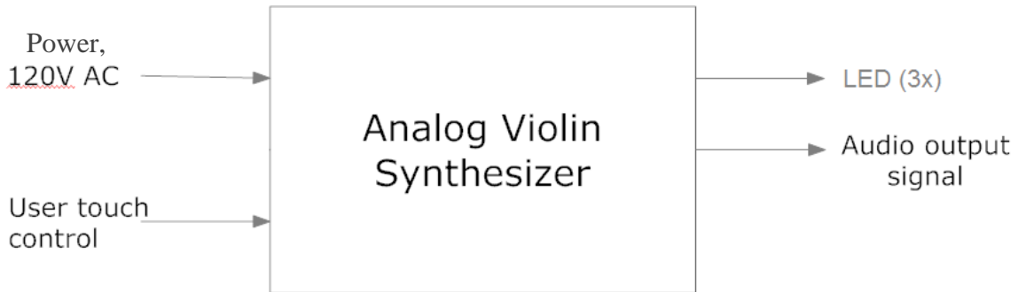
FIGURE 4 ANALOG VIOLIN SYNTHESIZER LEVEL 0 BLOCK DIAGRAM
