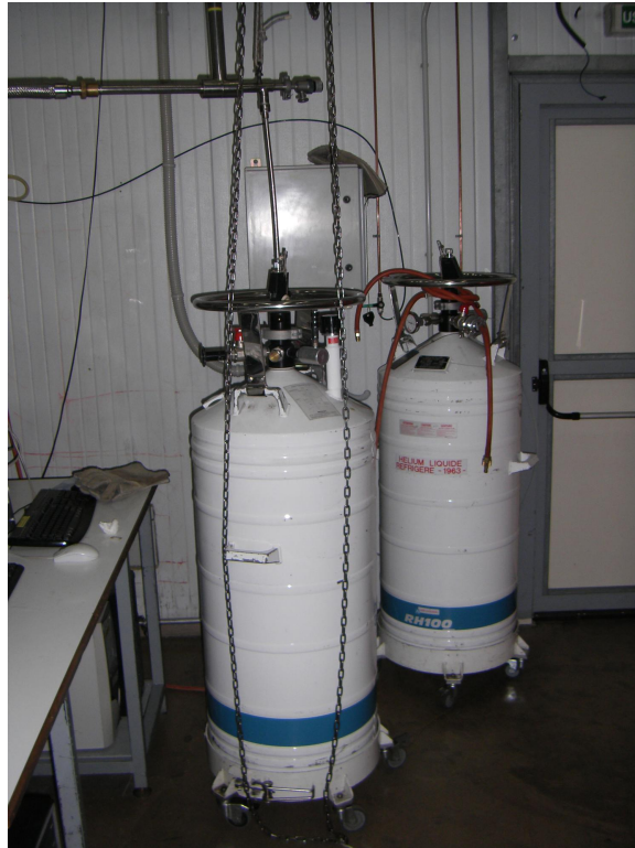
Figure 3: Liquid helium dewar being used to fill the main bath. The pipe coming out of the top is connected to the top of the cryostat which allows the main bath to be filled.
