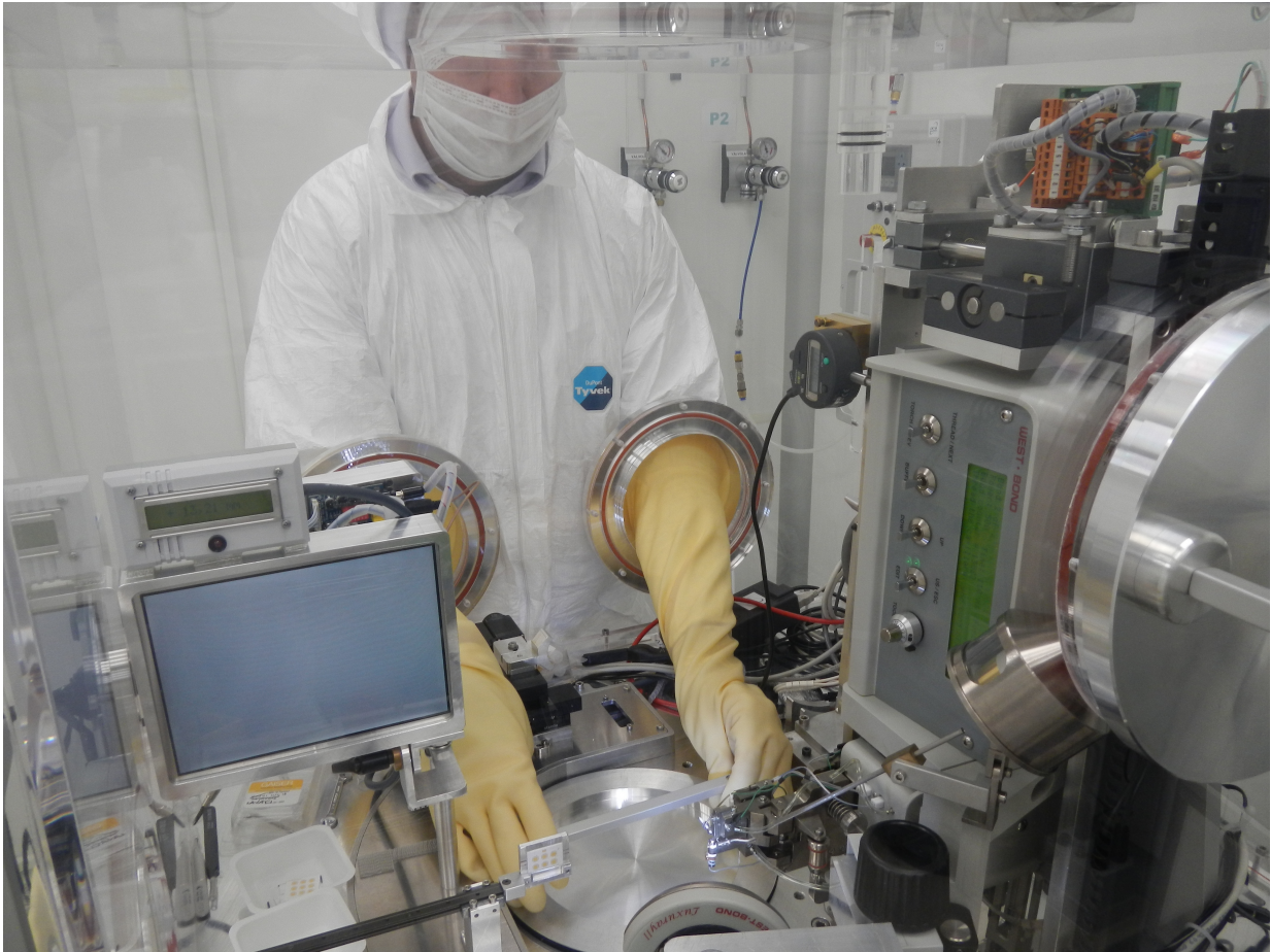
Figure 5: Changing a blocked capillary inside the glove box. The tower has been lowered into its housing.
