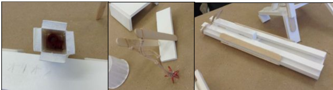
Figure 6 - Our Shooter Mechanism Concepts From Left to Right: Spring Tube, Pendulum, and Slide Track
