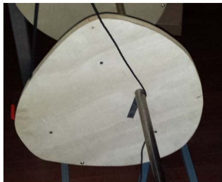
Figure 21 - Cam attached by bracket to the shaft
