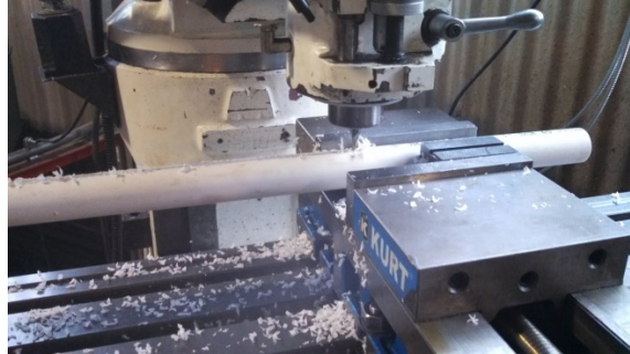
Figure 24 - Milling the PVC pipe
