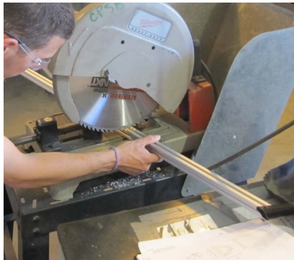
Figure 19 - Cutting an angled piece of frame
