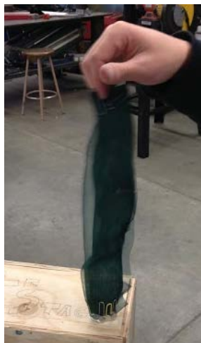
Figure 13 - Weighted fabric to simulate a swaying motion
