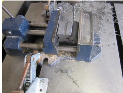
Figure 22 - Drilling a side-hole into a shuttle
