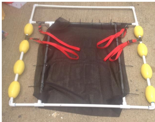
Figure 6.2 - Frame for day one of buoyancy testing
