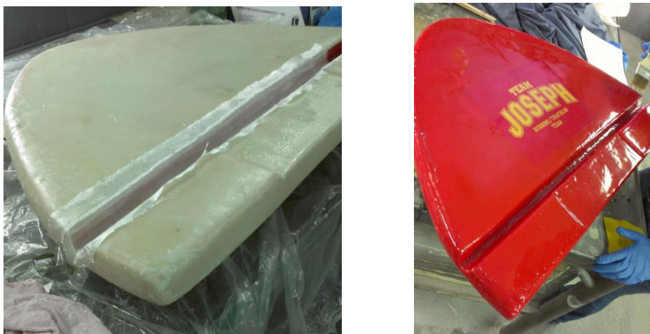
Figure 5.8 - The bow during fiberglassing and after final hot coat was applied
