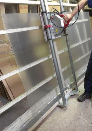
Figure 5.20 - Cutting the 4'x8' PETG sheet
