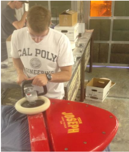
Figure 5.13 - Polishing the top of the bow
