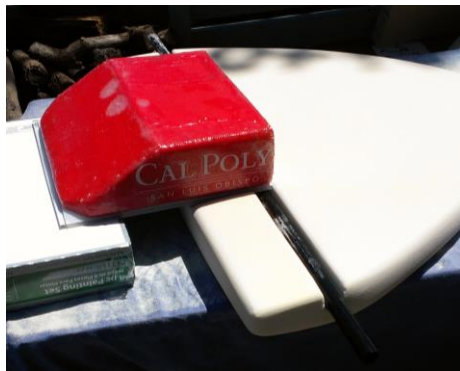
Figure 5.3 - Initial headrest before second hot coat was applied
