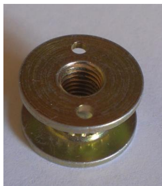
Figure 5.10 - Composite insert used to screw the splashguard to the bow
