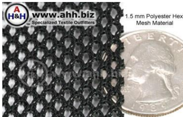
Figure 4.10 - Polyester hex mesh – zoomed in image displaying 1.5mm gage
