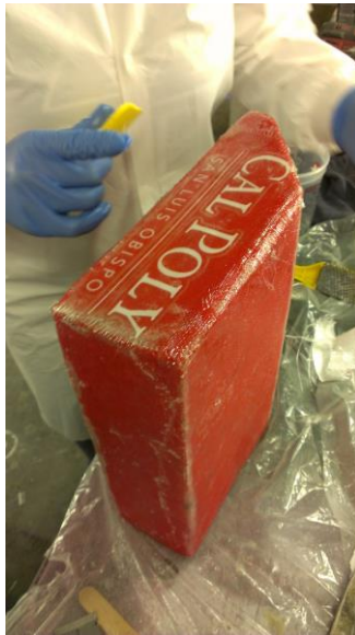
Figure 5.5 - One of the errors that was encountered was applying the sticker underneath the hot coat.
