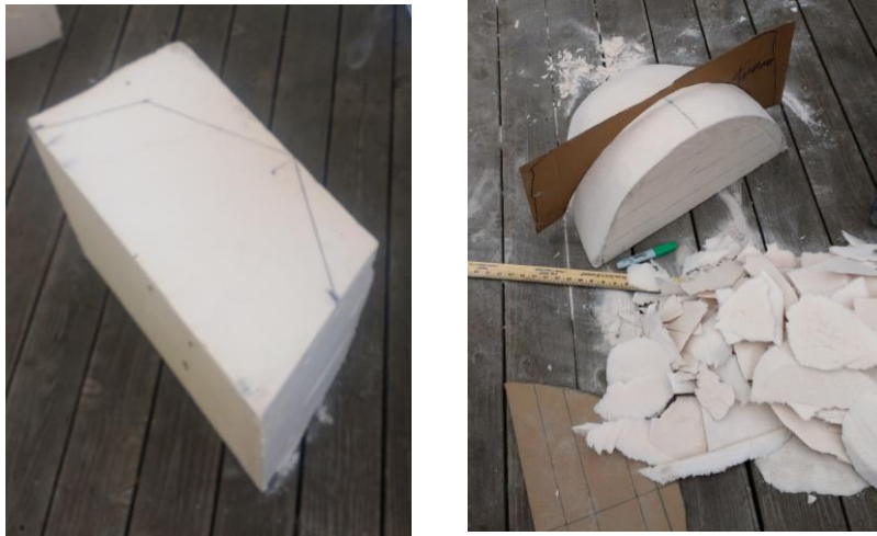
Figure 5.15 - Shaping the splashguard mold
