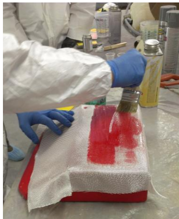
Figure 5.2 - Fiberglassing the headrest
