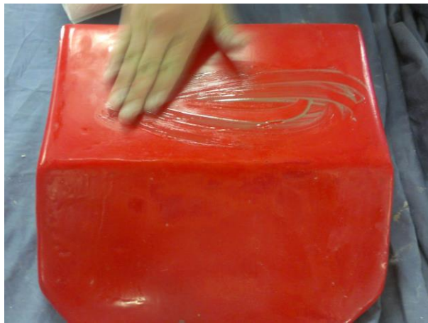
Figure 5.4 - Applying the final polishing compound to the headrest
