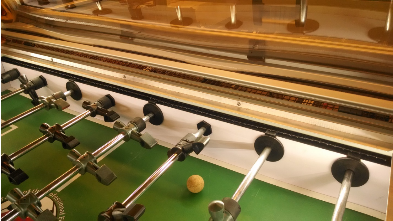
Figure 44. The aluminum sills block the blinding LEDs when the view is from above
