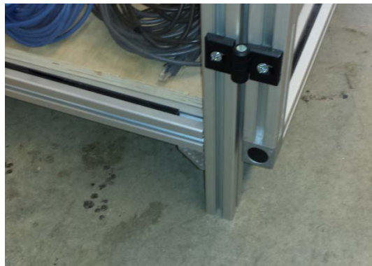
Figure 22: Current feet on the motor cabinet.
