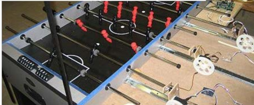
Figure 4: The foosball table made by the Georgia Institute of Technology. The gearing used to drive the rods can be seen.
