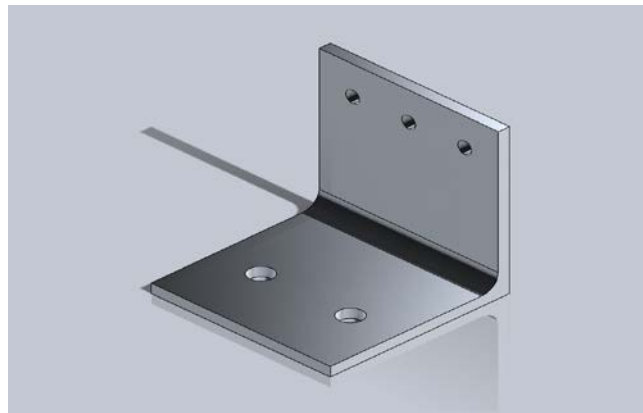
Figure 25: A solid works model of the bracket which will be mounted to the left side of the motor cabinet.
