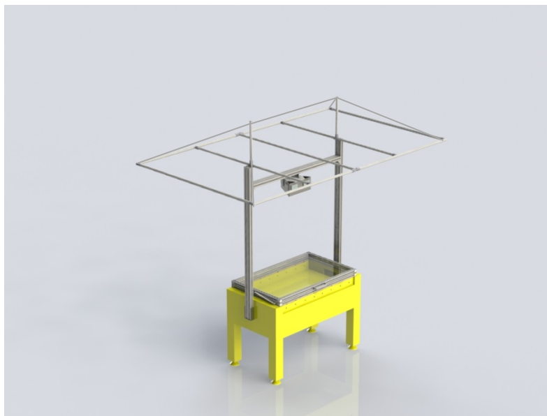
Figure 42. Final Roof, table, and playfield cover design
