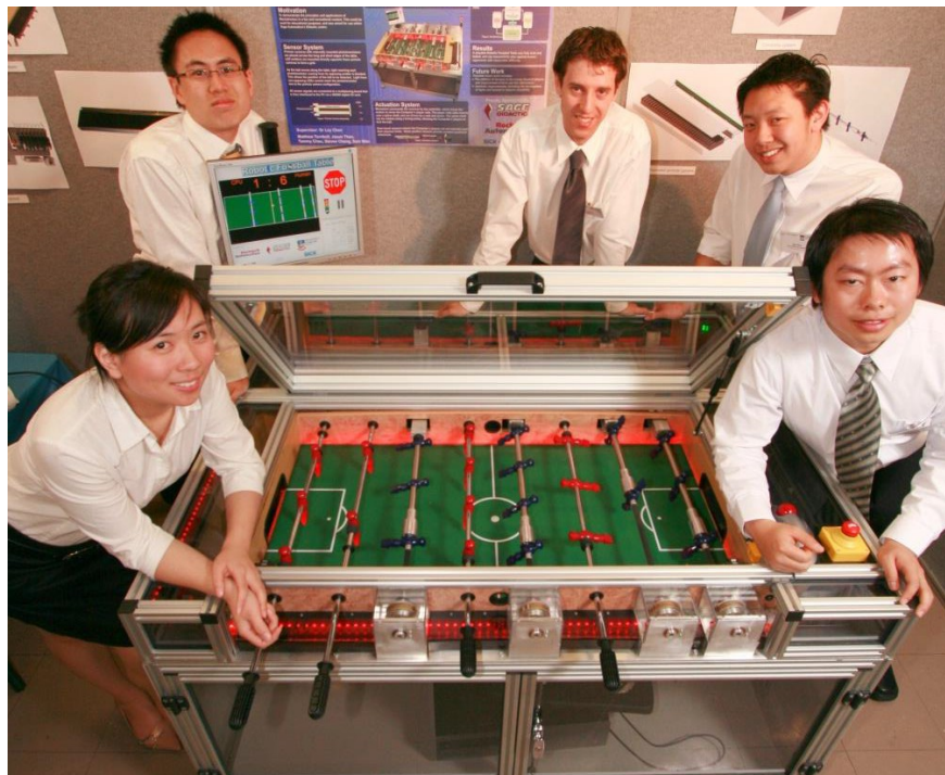
Figure 2: Robotic Foosball Table From the University of Adelaide, Australia.
