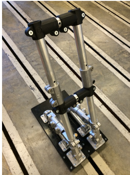
Figure 42: Test Stand Mounted to Strong Floor
