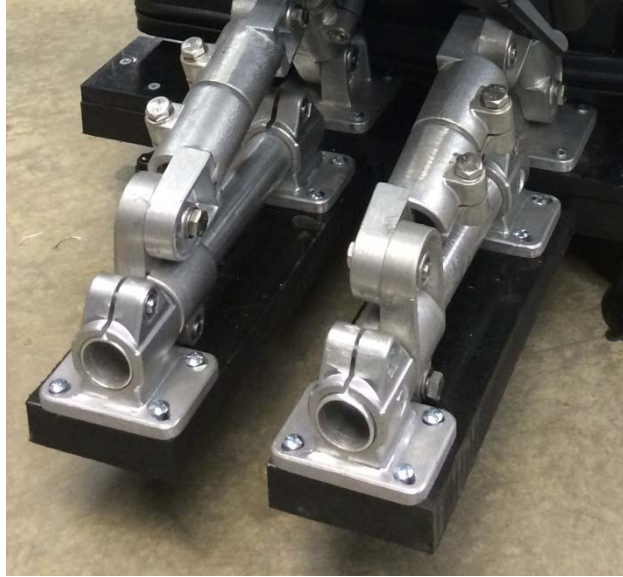
Figure 34: Joints Bolted to Seat Frame
