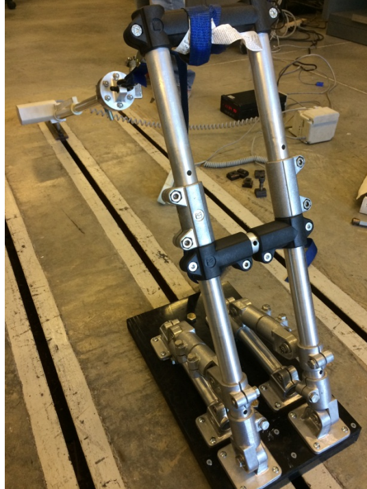
Figure 43: Test Setup with Actuator and Load Cell
