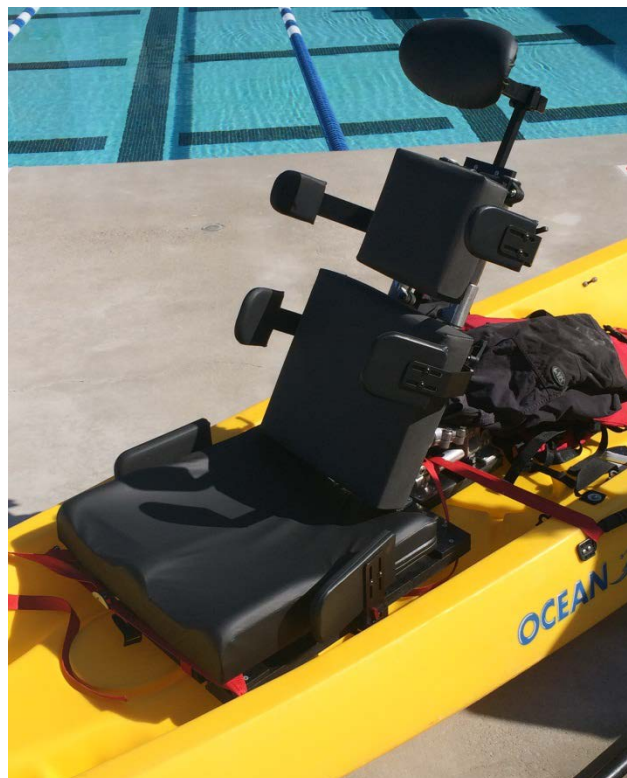
Figure 41: Modified Seat Attachment to Malibu II
