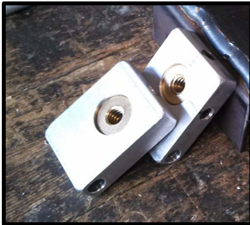
Figure 43. Lead screw hinges with the ACME nut imbedded
