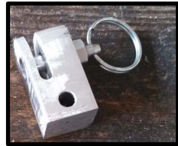
Figure 45. Release bracket, freshly milled and tapped, with the pull pin installed.
