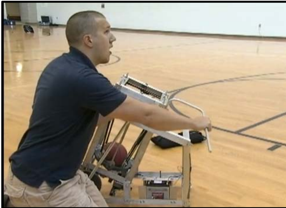
Figure 3. An Ohio University mechanical engineering student tests the team's basketball launcher.
