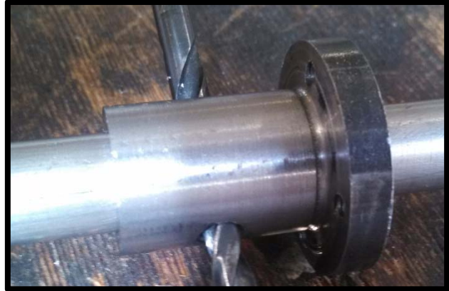
Figure 36. The ratchet flange attaches to the winch shaft via a set screw.
