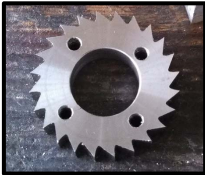
Figure 37. To attach the ratchet gear to its flange, four holes were milled and threaded.
