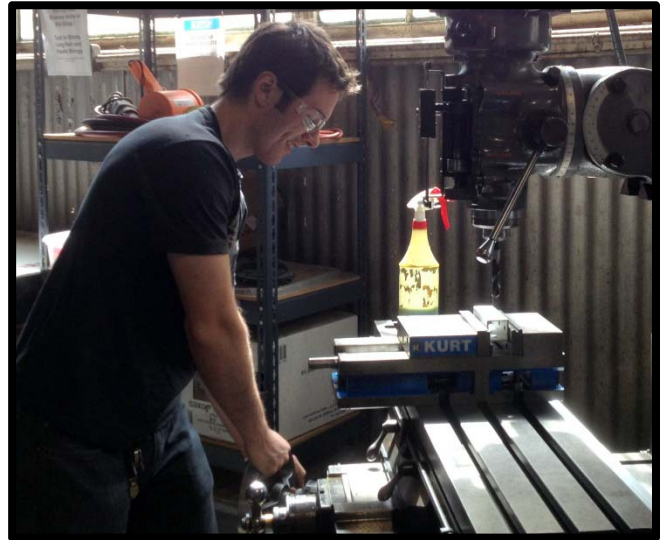
Figure 32. In order to drill precise holes in our frame members, the mill was used.
