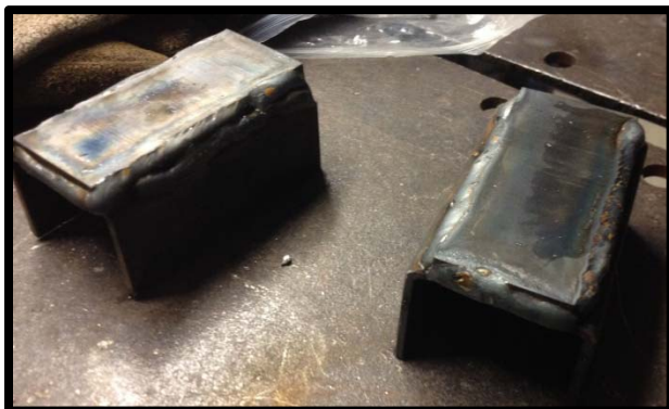
Figure 34. The steel rectangle was Mig welded to the custom u-channel.
