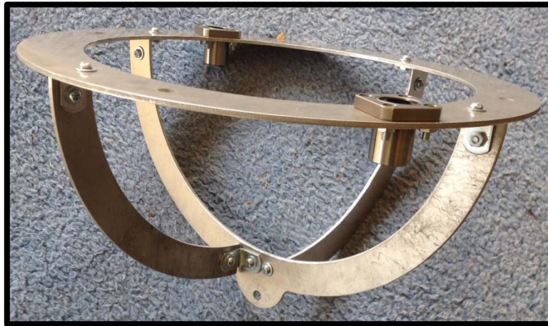
Figure 41. The carriage pieces were cut and bolted together with L-brackets
