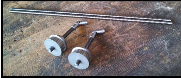
Figure 42. U-joints attached to the pulley shafts, and the lead screws above them
