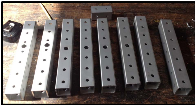
Figure 33. All short frame members cut to length with holes drilled.
